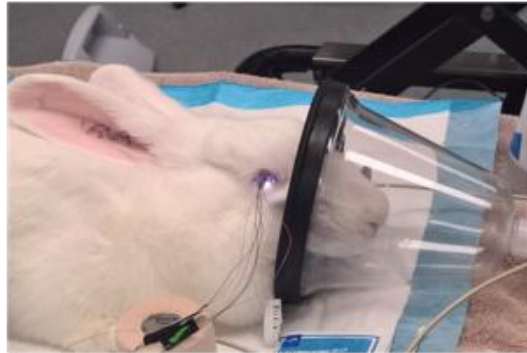
Figure 3. Anesthetized New Zealand white rabbit outfitted with the functioning and illuminated pupillometer during a test trial.
