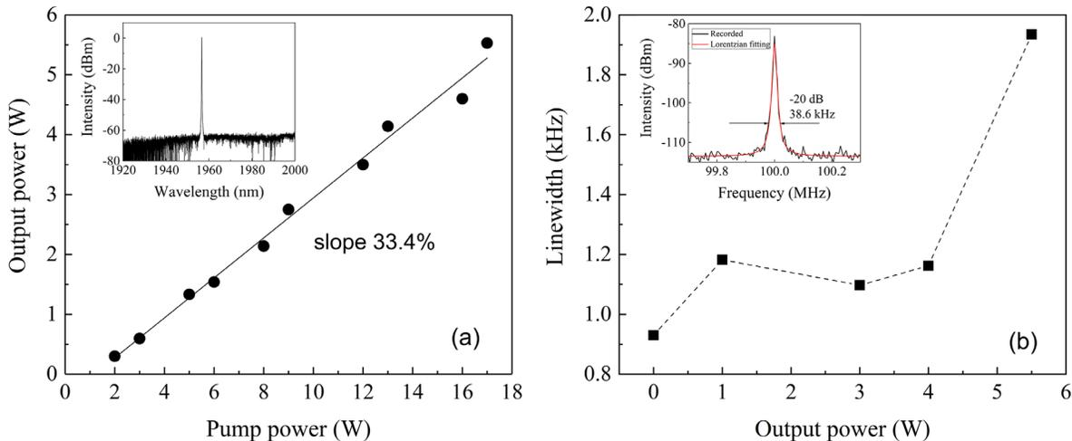
Figure 5. (a) Power transfer of amplifier; inset: spectrum recorded by the OSA Yokogawa 6375 at maximum power of 5.5 W. (b) Linewidth evolution of amplifier; inset linewidth measurement at maximum power of 5.5 W. The dashed lines serve as a visual guide.
