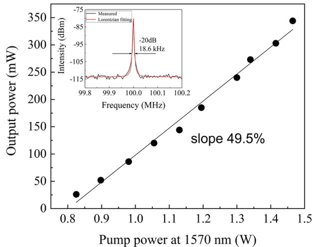
Figure 4. Power transfer of BTFL with 14-m-long cavity; inset: Stokes linewidth was measured at maximum output power of 344 mW. The dashed lines serve as a visual guide.
