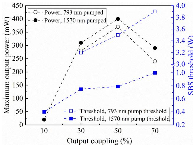
Figure 2. SBS threshold and Stokes output power with different output coupling under fixed Brillouin pump of 250 mW
