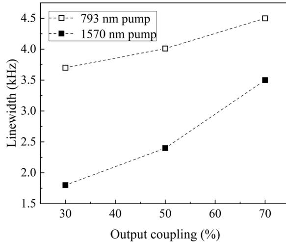
Figure 3. Stokes BTFL linewidths measured with different coupling and pump schemes. The dashed lines serve as a visual guide.
