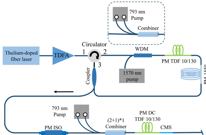
Figure 1. Schematic of hybrid Brillouin/thulium fiber laser.
