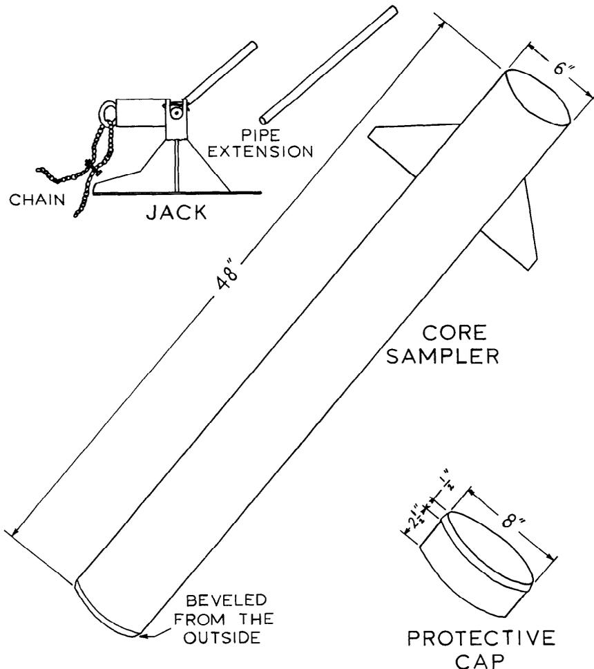
FIGURE 1. Sketch showing the construction of a simple core sampling device, its protective cap, and the jack for removal of cores from the soil.
