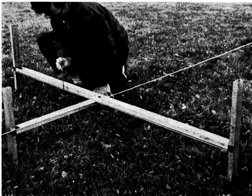
FIGURE 1. The T-frame in normal position relative to the 100-foot measuring tape with a loop-position measurement being recorded. The tape bisects the cross member and lies flush to the axial member of the T-frame.
