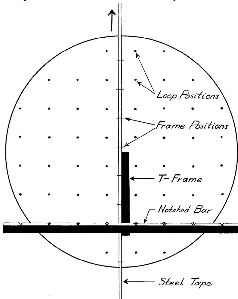
FIGURE 3. Schematic diagram showing relation of plot, measuring tape, T-frame, and the 50 loop positions. The frame is shown alined at the second position.
