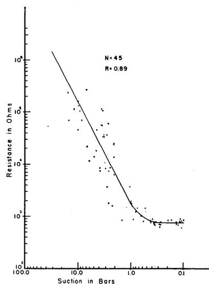
FIGURE 1. Calibration curve for Bouyoucos resin impregnated gypsum blocks.
