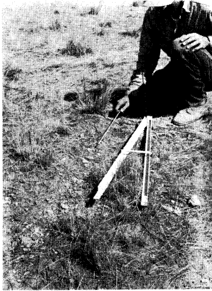
FIGURE 1. An acute angle was prepared by welding 1½-inch angle iron and drilling a ¼-inch hole at the vertex.
