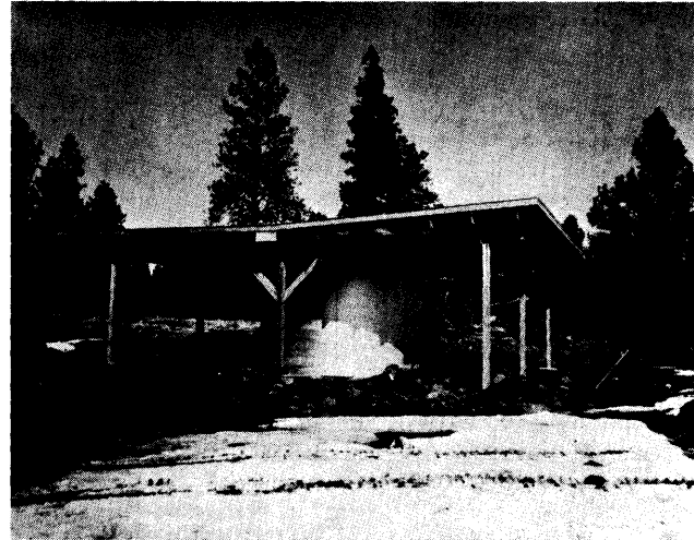
FIG. 1. Intermediate-size (8,600 gal) trick tank for storing livestock drinking water.
