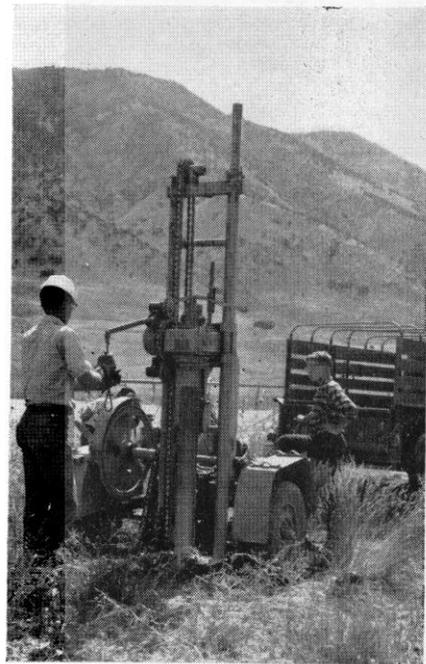
FIGURE 1. The Kelly Core Sampler in operation. The core is approximately two feet down in the soil. One man can operate it efficiently although two may be needed to handle the core after extraction.
