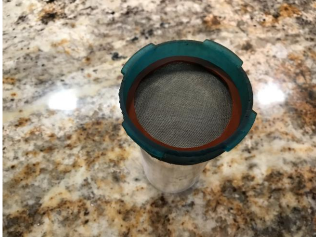
Figure K: Filter in filter housing (quarter turn locking method shown), secured by o-ring
