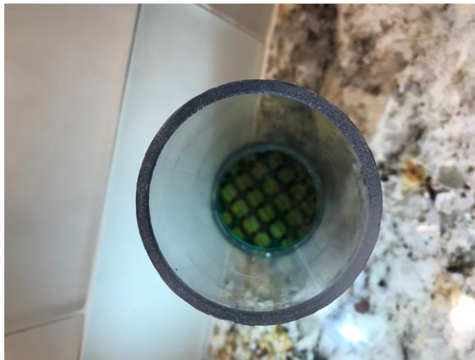
Figure D: Top view of static mixing grid in attachment
