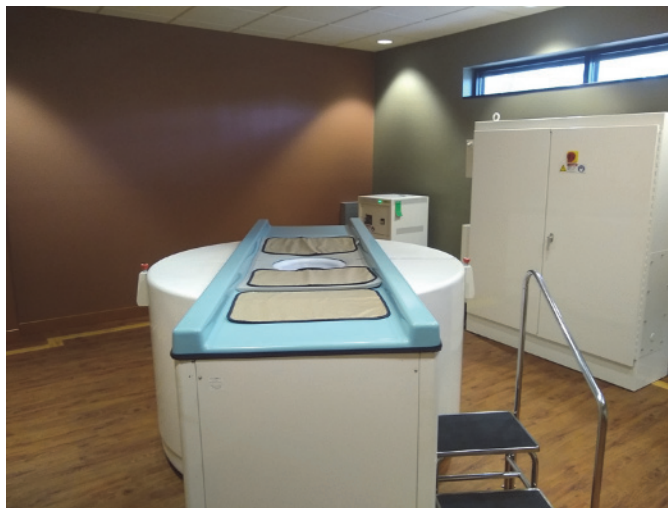
Fig 1. Photograph of the dedicated cone-beam breast CT system employing offset detector geometry.
