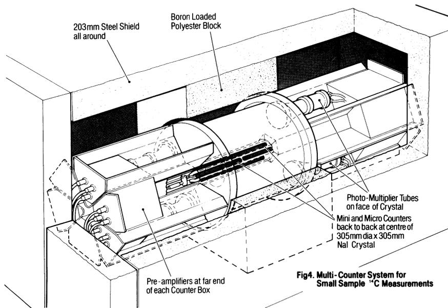
Fig 1. Multi-counter system for small sample  $^{14}\text{C}$  measurements
