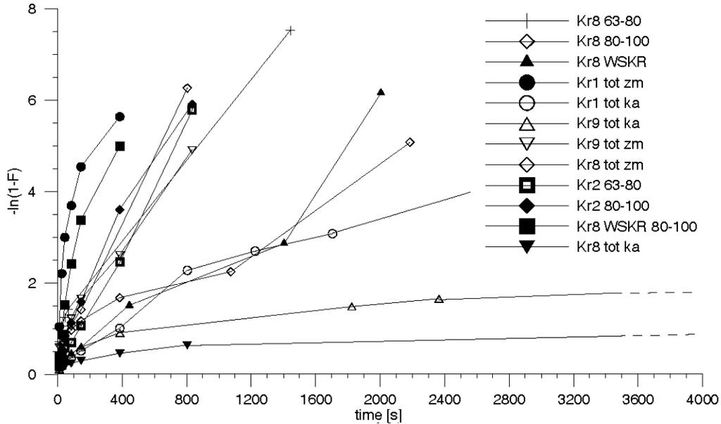
Figure 4 Leaching reaction of different fractions of mortar samples from the Small Scales in Kraków (descriptions of the fractions are given in the text). Like in Figure 2, the cumulative CO<sub>2</sub> pressure is represented by  $-\ln(1-F)$ .
