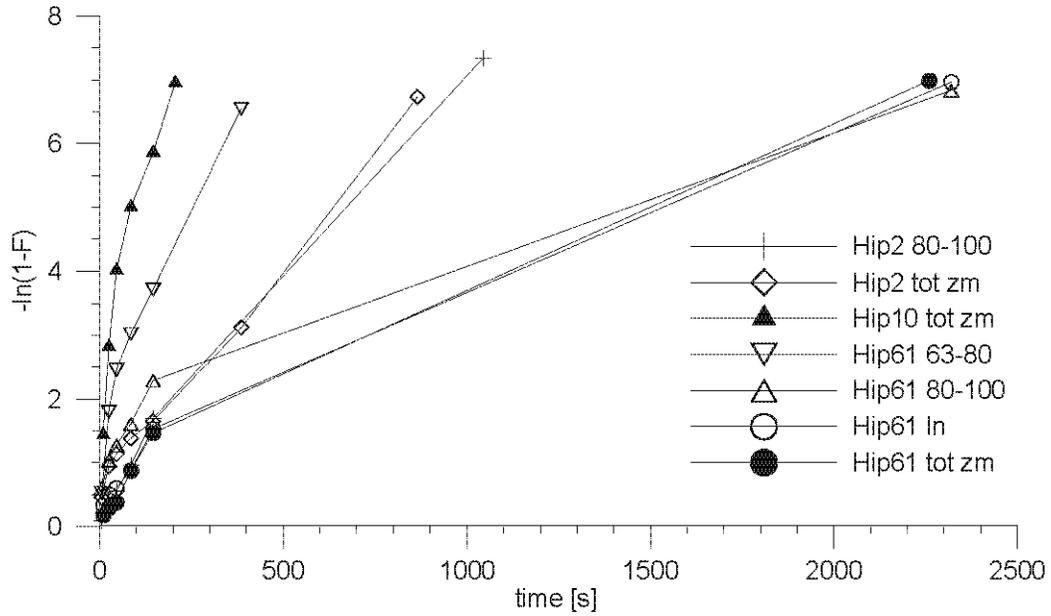
Figure 2 Leaching reaction of different samples from the NW Church in Hippos. Cumulative CO<sub>2</sub> pressure is represented by  $-\ln(1-F)$ , where  $F = p/p_{tot}$  and plotted versus time, and  $p_{tot}$  is the pressure of CO<sub>2</sub> at the end of the reaction.
