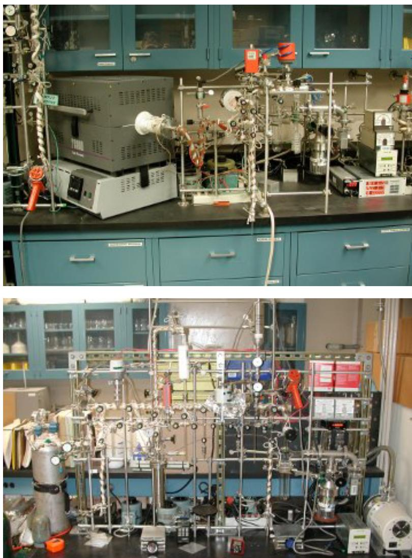
Figure 2 Photographs of the modified extraction line (upper panel) and CO<sub>2</sub> purification line (lower panel). All glass tubing (except coil traps and cold fingers) and glass-metal connections are covered by heat tape that is maintained at 50–70 °C to minimize gas adsorption inside the line.
