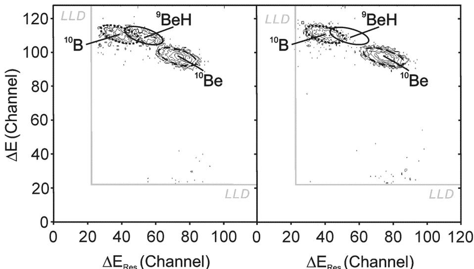
Figure 1 Left: spectrum of a <sup>10</sup>Be standard in charge state 2+ and for a stripper gas pressure of 0.3 μg/cm<sup>2</sup> (optimum for maximal transmission of <sup>9</sup>Be+). A (<sup>9</sup>BeH)<sup>2+</sup> peak shows between <sup>10</sup>B<sup>2+</sup> and <sup>10</sup>Be<sup>2+</sup>. The (<sup>9</sup>BeH)<sup>2+</sup> can be eliminated if the gas pressure is raised to 1 μg/cm<sup>2</sup> (shown on the right).
