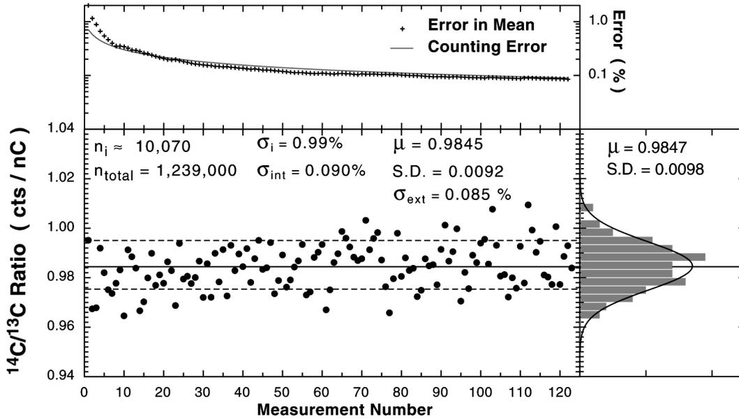
Figure 1 Sequential measurements of a sample of ANU sucrose (1.5 Modern) were distributed normally with a standard deviation equal to the counting statistics of the individual measurements ( $\sigma_i$ ). The standard error in the mean of the distribution,  $\sigma_{ext} = 0.085\%$ , was smaller than the total counting statistics of the entire data set (0.090%).
