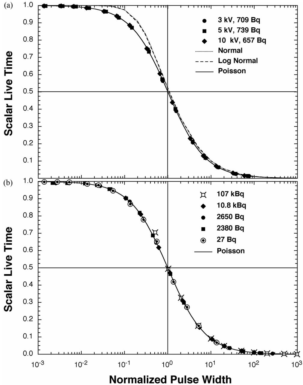
Figure 4 (a) The scalar live time follows the same function of normalized pulse width for 3 different cesium sputtering energies. The function is best described by a Monte Carlo simulation assuming a Poisson distribution of ion arrival times; (b) The same function of live time is found for a range of mean count rates from 27 to 107,000 counts per second.
