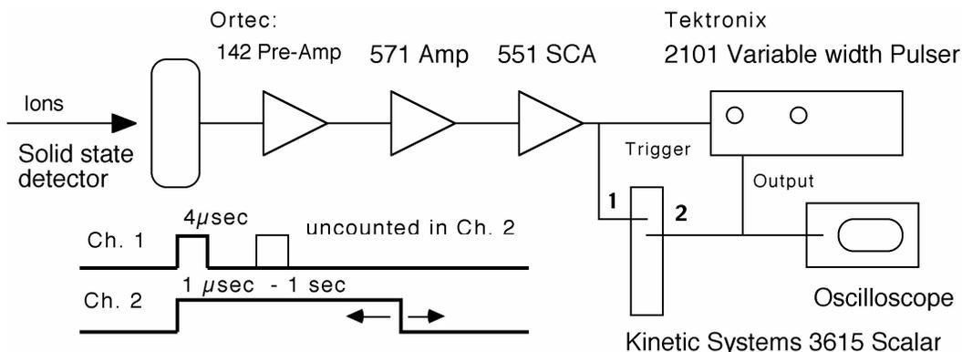
Figure 3 Apparatus for determining the dependence of scalar live time on the ion arrival time distribution
