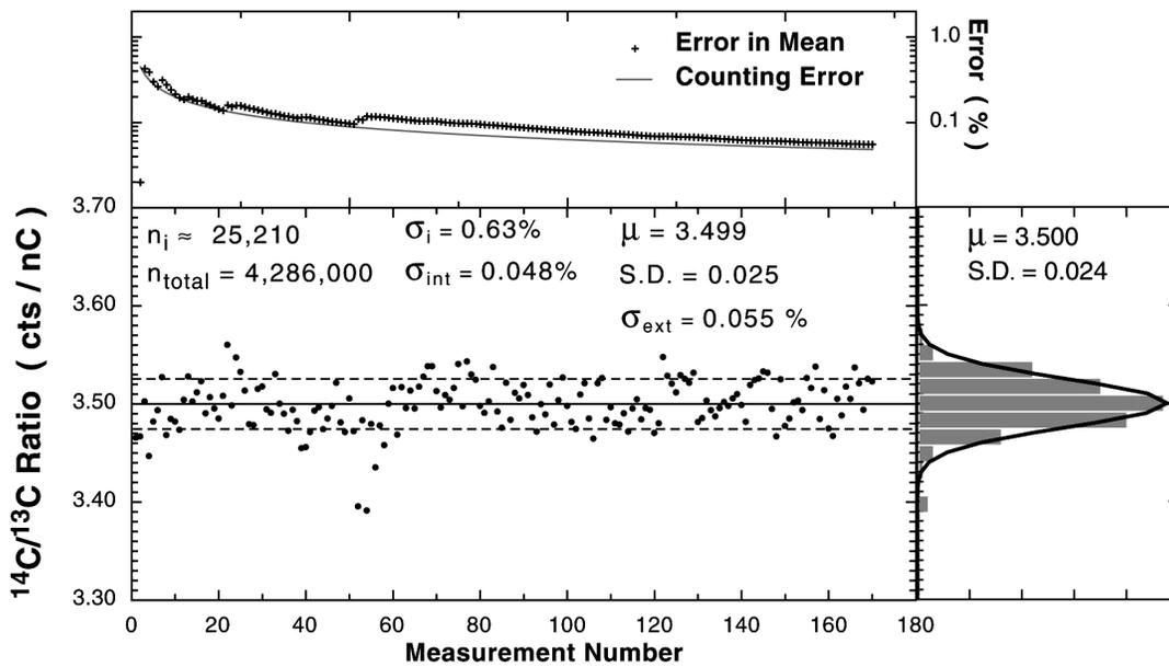
Figure 2 Sequential measurements of a sample of a 5 Modern sample were distributed normally with a standard deviation slightly larger than the counting statistics of the individual measurements ( $\sigma_i$ ). The standard error in the mean of the distribution,  $\sigma_{ext} = 0.055\%$ , was similar to the total counting statistics of the entire data set (0.048%).
