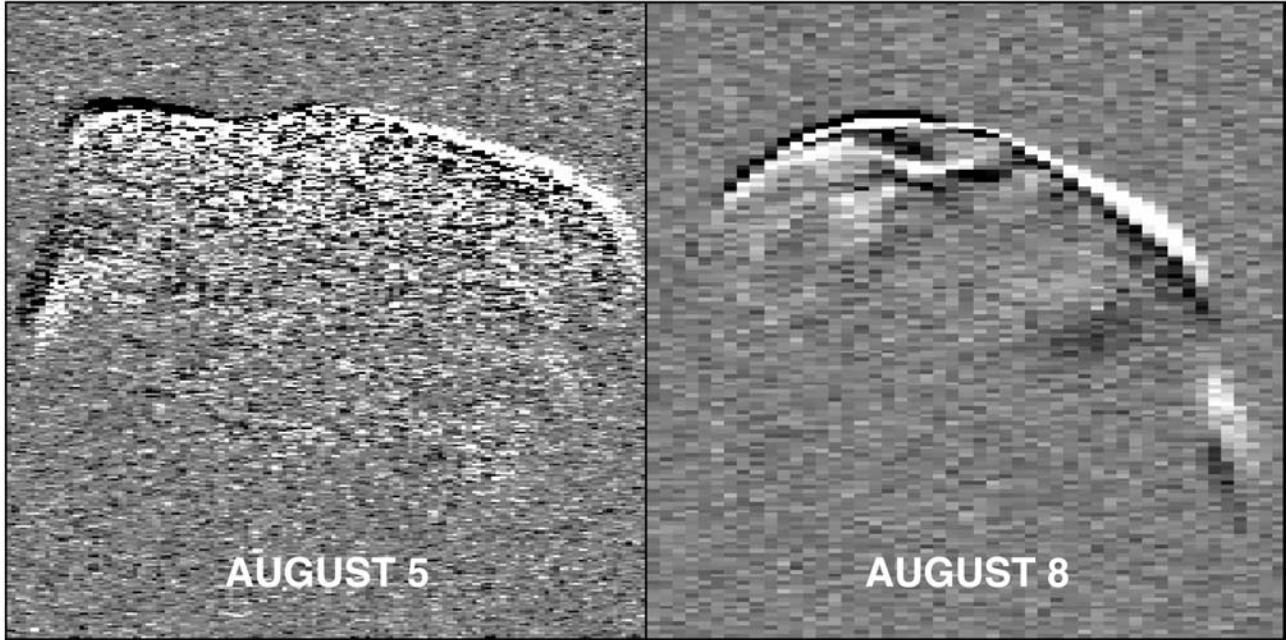
FIG. 3. Difference images obtained on August 5 (left) and 8 (right), the longest tracks at Arecibo and Goldstone. Range increases from top to bottom and Doppler frequency increases from right to left, so rotation is clockwise. The August 5 (Arecibo) image shows the difference between the first (white) and last (black) runs on that day, which were obtained 1.3 h apart. The August 8 (Goldstone) image shows the difference between the first 17 runs (white) and the last 14 runs (black), which were obtained 7.5 h apart. Several degrees of rotation are evident in the August 8 image.
