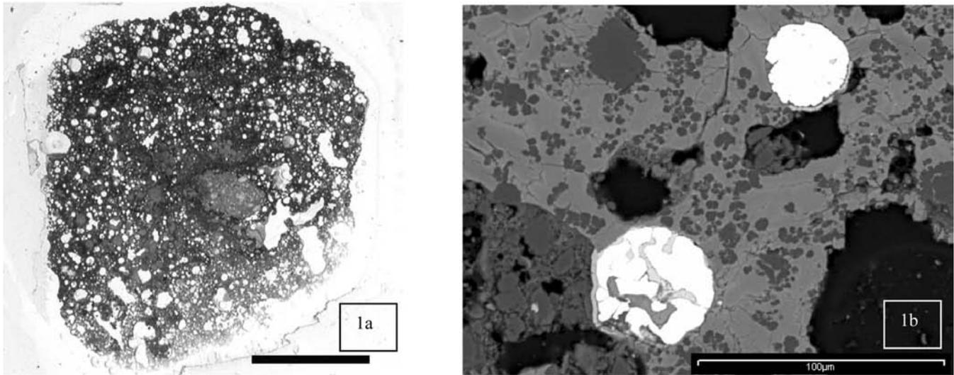
Fig. 1. a) Transmitted light photograph of a polished section of vesicular glass in a cm-scale melt droplet. Vesicles appear pale, and a clast of shocked but unmelted calcite-cemented sandstone is visible near the center. The scale bar is 5 mm; b) backscattered electron image (BEI) of a typical area of the Barringer melt droplet. The white is nickel- and cobalt-rich metal, the pale grey is glass and calcic clinopyroxene, and the dark grey is silica. The scale bar is 100  $\mu\text{m}$ .
