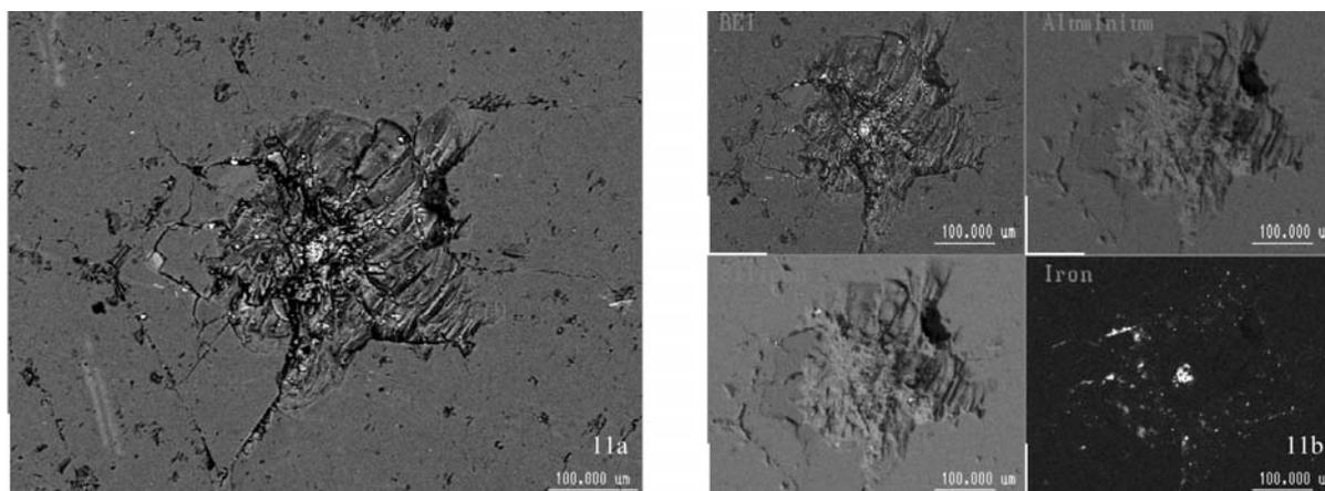
Fig. 11. a) BEI of crater on a polished surface of feldspathic gneiss, generated by impact of a small kamacite particle (38–58  $\mu\text{m}$  diameter) moving at  $\sim 5 \text{ km s}^{-1}$  in a light gas gun. The scale bar is 100  $\mu\text{m}$ ; b) EDS X-ray maps of an enlarged central area show concentration of projectile metal melt within the central pit and dispersion of brecciated target sulfide grains along radial fractures. The scale bar is 100  $\mu\text{m}$ .
