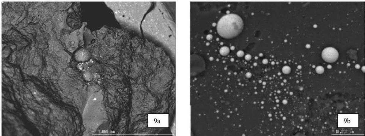
Fig. 9. a) BEI of broken surface shows glassy and vesicular silicate melt vein cutting breccia. The bright spots are metal. The scale bar is 1 mm; b) BEI of interior of vesicle in melt vein shows metal droplets of diverse size but apparently identical composition. The scale bar is 10  $\mu\text{m}$ .
