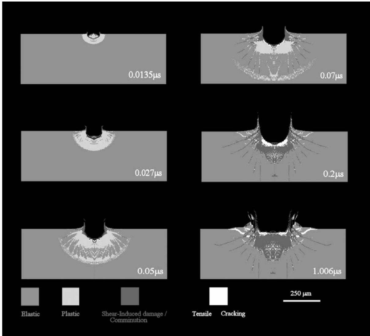
Fig. 12. Six timed frames from an AUTODYN-2D impact simulation of the first microsecond following contact of a 50  $\mu\text{m}$ -diameter glass sphere moving at 4  $\text{km s}^{-1}$  perpendicular to a glass surface (for more details of this simulation, see McDonnell et al. [2001]). The material state is described by color code. Note early strain localization and generation of well-defined zones of shear comminution and slightly later tensile cracking. The scale bar is 250  $\mu\text{m}$ .
