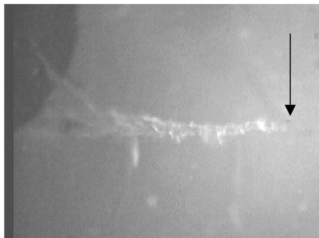
Fig. 1. A typical track in aerogel (side view). An impact of rhodonite in aerogel (density 60 kg m -3 ) at 5.1 km s -1 . Track length is 3.6 mm and particle size is 54 microns. The impact was from the left; the particle position is marked with an arrow.
