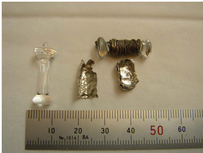
Fig. 1. Experimental setup used for the in vacuo removal of sulfur from the decomposition of troilite during step heating analysis. The coil and the quartz rod on which the Fe wire is wrapped (see text) are shown (mm scale). Evidence for reaction of sulfur vapor with Fe wire is apparent. The Pt sample boat is used as a container for in vacuo transfer of troilite chips, without the troilite chips coming in contact with the quartz glass.
