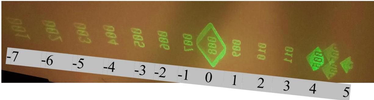
Figure 7. Observation screen of ASLM output by a DLP7000 DMD using all output diffraction orders across the  $+12^\circ$  and  $-12^\circ$  micromirror span. The projected patterns have reversed parity.
