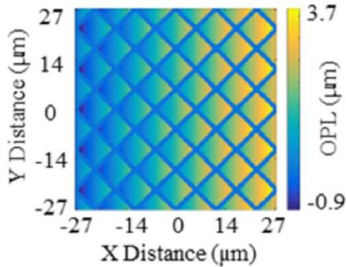
Figure 1. Phase map of a 5×5 array of 10.8 μm corner-to-corner pitch micromirrors with 3° angle-of-incidence illumination. The micromirrors shown are fixed at -12° relative to the DMD structure surface. Reprinted<sup>6</sup>.
