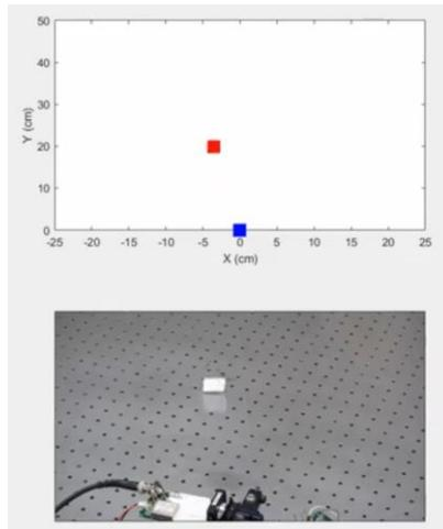
Figure 3. Lidar capture (top) and experimental setup with target (bottom). Reprinted<sup>6</sup>.
