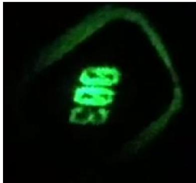
Figure 8. Direct viewing of the DLP7000. Oversaturation of the photo reduced image quality significantly, but full DLP7000 resolution is available.
