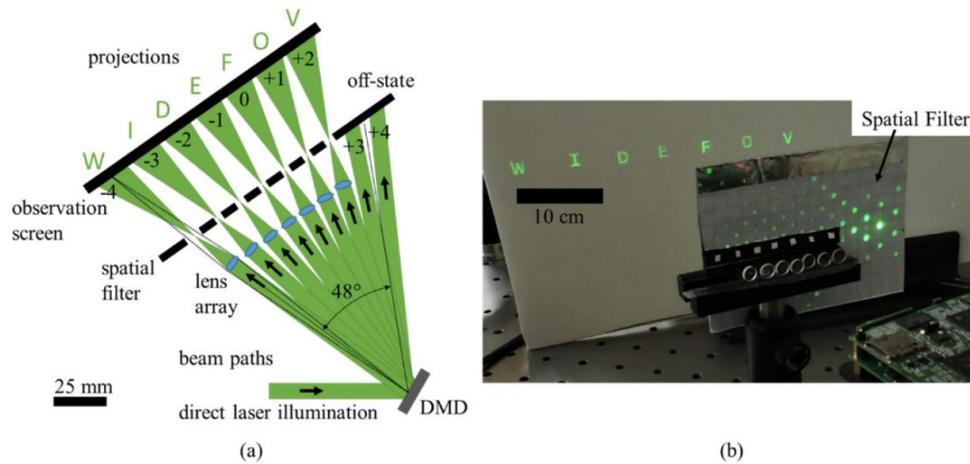
Figure 5. ASLM extended display including (a) schematic depiction and (b) experimental result. Reprinted<sup>7</sup>.
