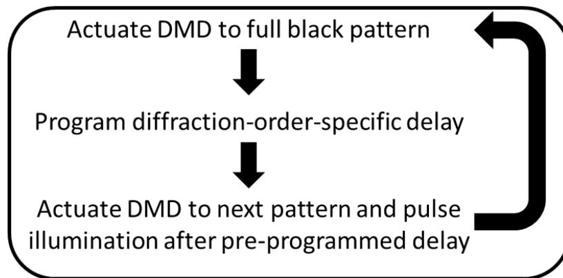
Figure 4. ASLM pattern steering sequence.
