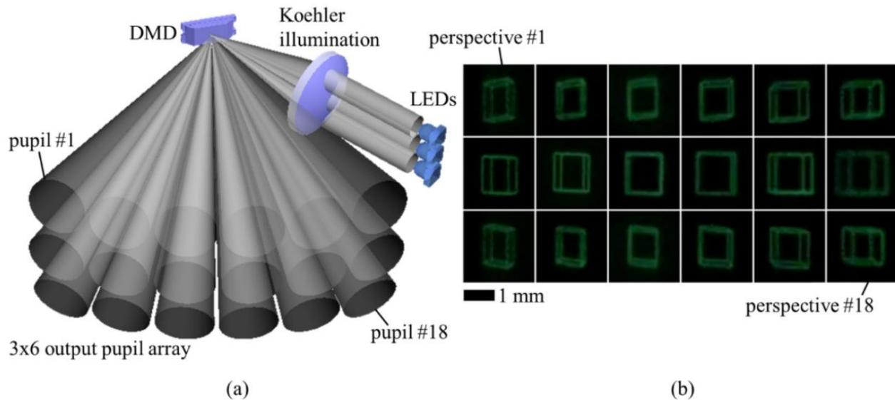
Figure 6. 2D pattern steering including (a) schematic depiction and (b) captured images of the 6×3 array perspectives. Reprinted<sup>7</sup>.
