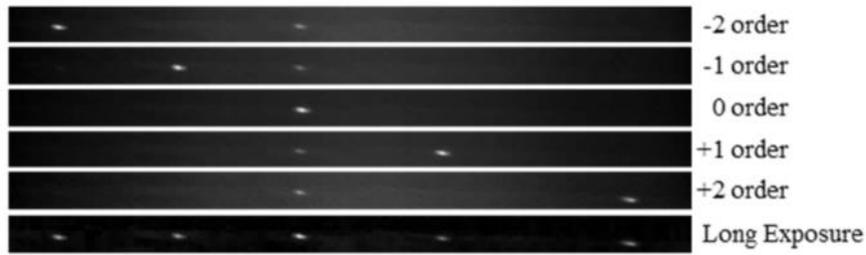
Figure 2. Discrete steering points across five output diffraction order directions. The 0<sup>th</sup> order diffraction order includes the cover glass reflection which is visible when steering the beam in any diffraction order. Reprinted<sup>6</sup>.
