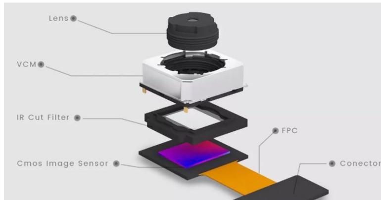
Fig. 2. Diagram of a camera module.<sup>1</sup>
