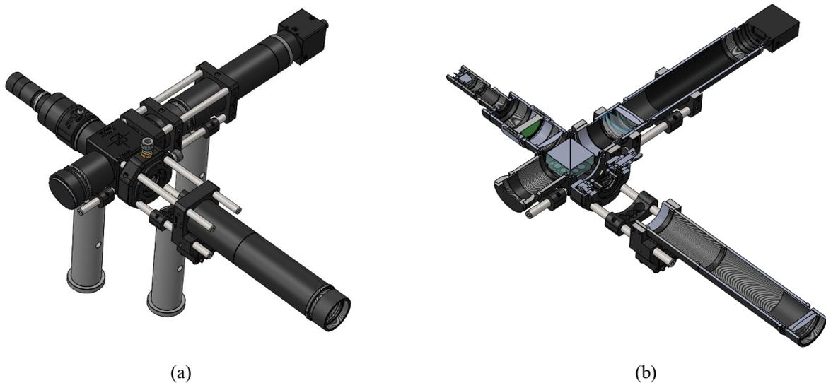
Fig. 9. A) Collimator assembly; and b) cutaway view.
