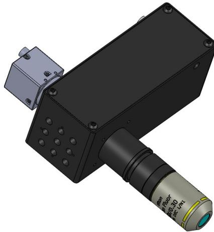
Fig. 10. W2-AM with Nikon objective attached. This is the microscope used to capture images in the focal plane of the test lens.
