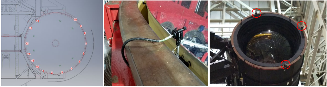
Figure 2 Primary mirror cell positions around the primary mirror (left). There are a total of 16 collimator mounts attached directly to the primary mirror using silicone sealant and Invar base to prevent damage to the primary mirror due to thermal expansion. The collimator mounts are then magnetically coupled to the mirror bases (center). There are 9 collimators aligned to retroreflectors on LBC. Three retroreflectors are installed on the outer rim of the LBC (right, red circles).
