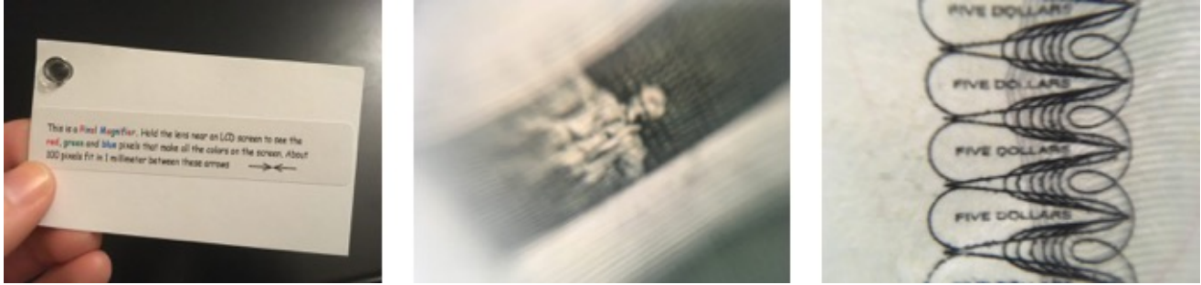
Figure 5. Left: Pixel viewer made from a business card and macro lens. Center and Right: Images of microprint on US currency as captured with a phone camera through the pixel viewer.
