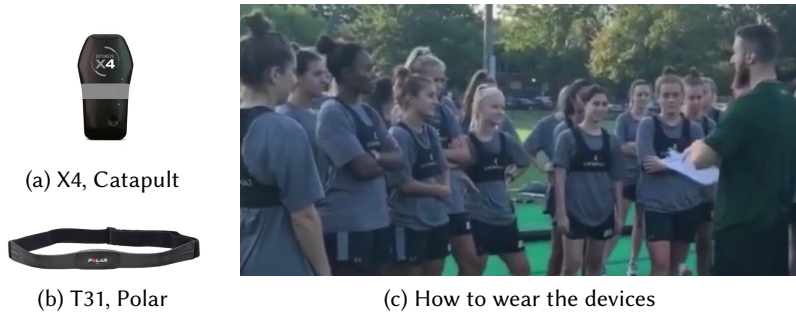
Fig. 6. Data Collection Devices — Each player wore X4 for IMU data and T31 for Heart Rate data.
