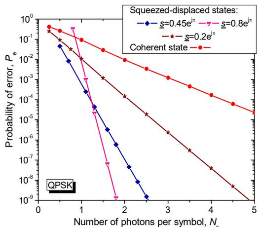
Fig. 1 Uncoded symbol error probability vs. average number of signal photons/symbol for squeezed-displaced states-based QPSK in the absence of noise.
