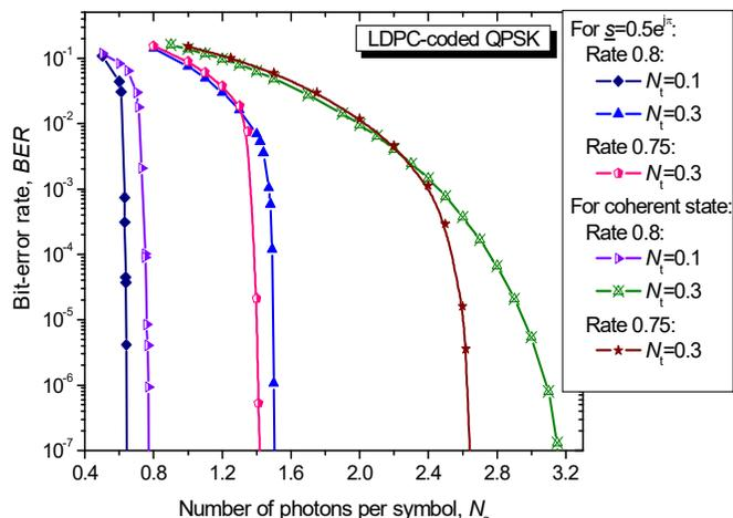
Fig. 2 BER performance of LDPC-coded squeezed-displaced states-based QPSK vs. average number of signal photons/symbol  $N_s$  for different average number of noise photons  $N_t$ .
