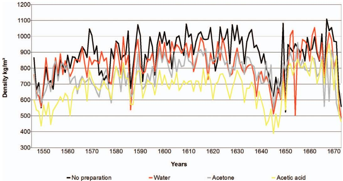
**Figure 2.** Example graph demonstrating maximum density values obtained for sample 117A before extraction, as well as after the application of consecutive reagents.
