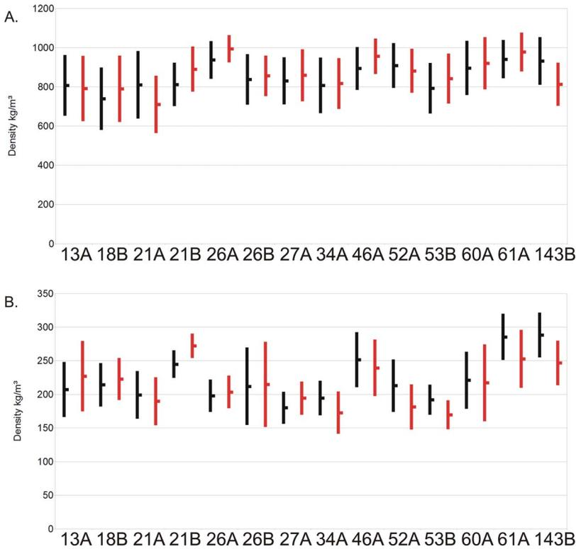
**Figure 4.** The values of maximum (a) and minimum (b) ring density averaged for particular samples before preparation (black) and after the application of cold de-ionized water (red). Middle point of each line represents the mean value and length of the line refers to standard deviation range.
