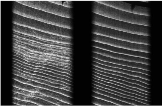
**Figure 5.** X-ray film presenting the creased zone of sample 117A before preparation and the same place smoothed after soaking in cold de-ionized water.
