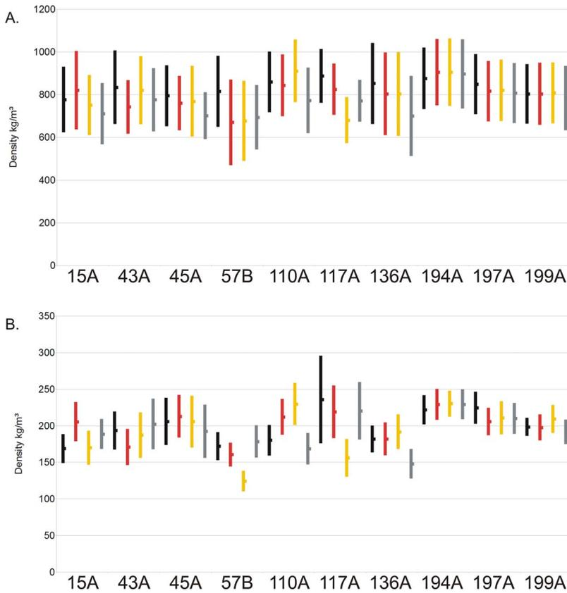
**Figure 3.** The values of maximum (a) and minimum (b) ring density averaged for particular samples before preparation (black) and after the application of hot de-ionized water (red), acetone (yellow) and diluted acetic acid (gray). Middle point of each line represents the mean value and length of the line refers to standard deviation range.
