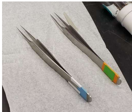
Figure 17. Forceps used for brain dissections, as well as adjusting the positioning of the brains when necessary during subsequent washing, blocking, staining, and mounting.
