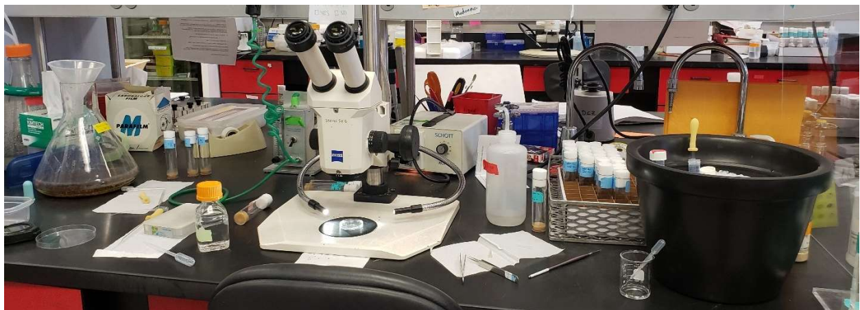
Figure 18. Dissection set-up. Petri dish is illuminated beneath the microscope; flies are knocked out on the CO 2 pad to the left, and fly brains are transferred to microcentrifuge tubes in the ice bath to the right. Forceps are placed on a Kim wipe when not in use to prevent contamination.
