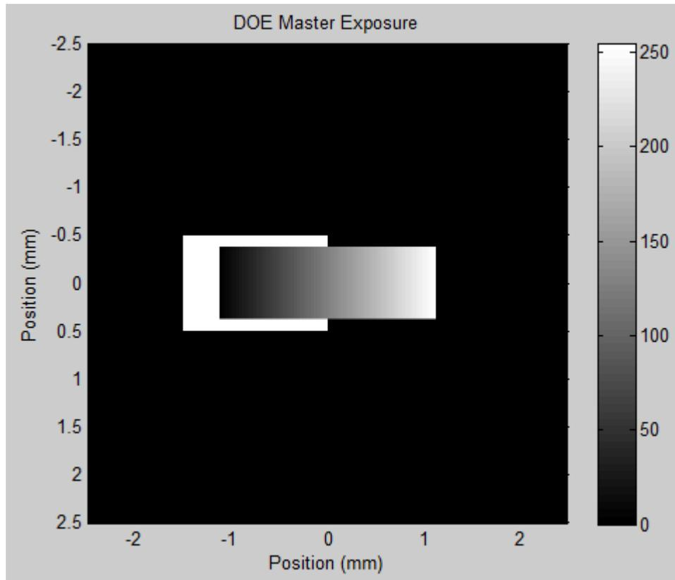
Figure 48 Example Ramp exposure pattern detailing a simple exposure ramp.
