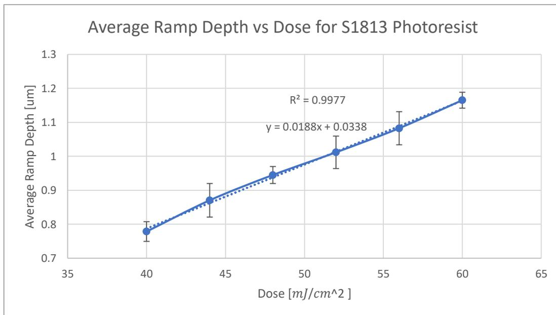
**Figure 21 Average ramp height vs dose plotted using the data shown in Table 3. A linear trendline is plotted with equation and R squared value shown. Error bars show +/- one standard deviation of the data set.**
