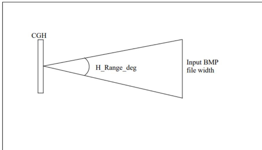
**Figure 25 Description of the Gerchberg-Saxton beam shaper element parameter  $H\_range\_deg$  [20]**
