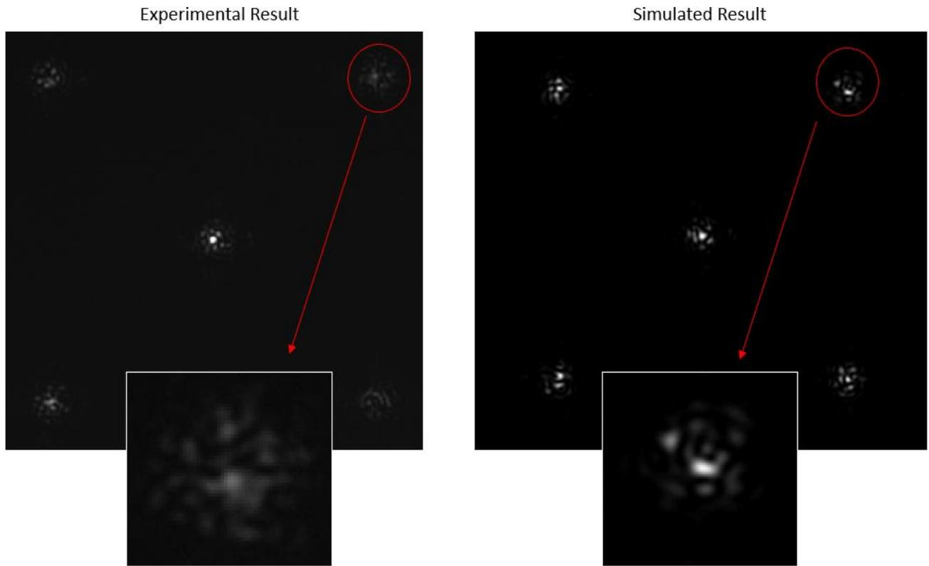
**Figure 43 Comparison of the experimental image of the CGH taking using the CGH testbed and the simulated result.**
