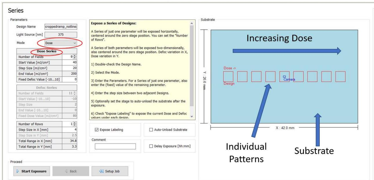
**Figure 19 Exposure start menu on the MLA 150 demonstrating the layout and configuration of a series dose test. The options for dose values are given on the left and the layout of the patterns on the substrate is demonstrated on the right.**
