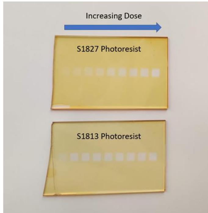
**Figure 20** Example comparison of S1813 and S1827 photoresist exposures after an increasing dose series exposure
