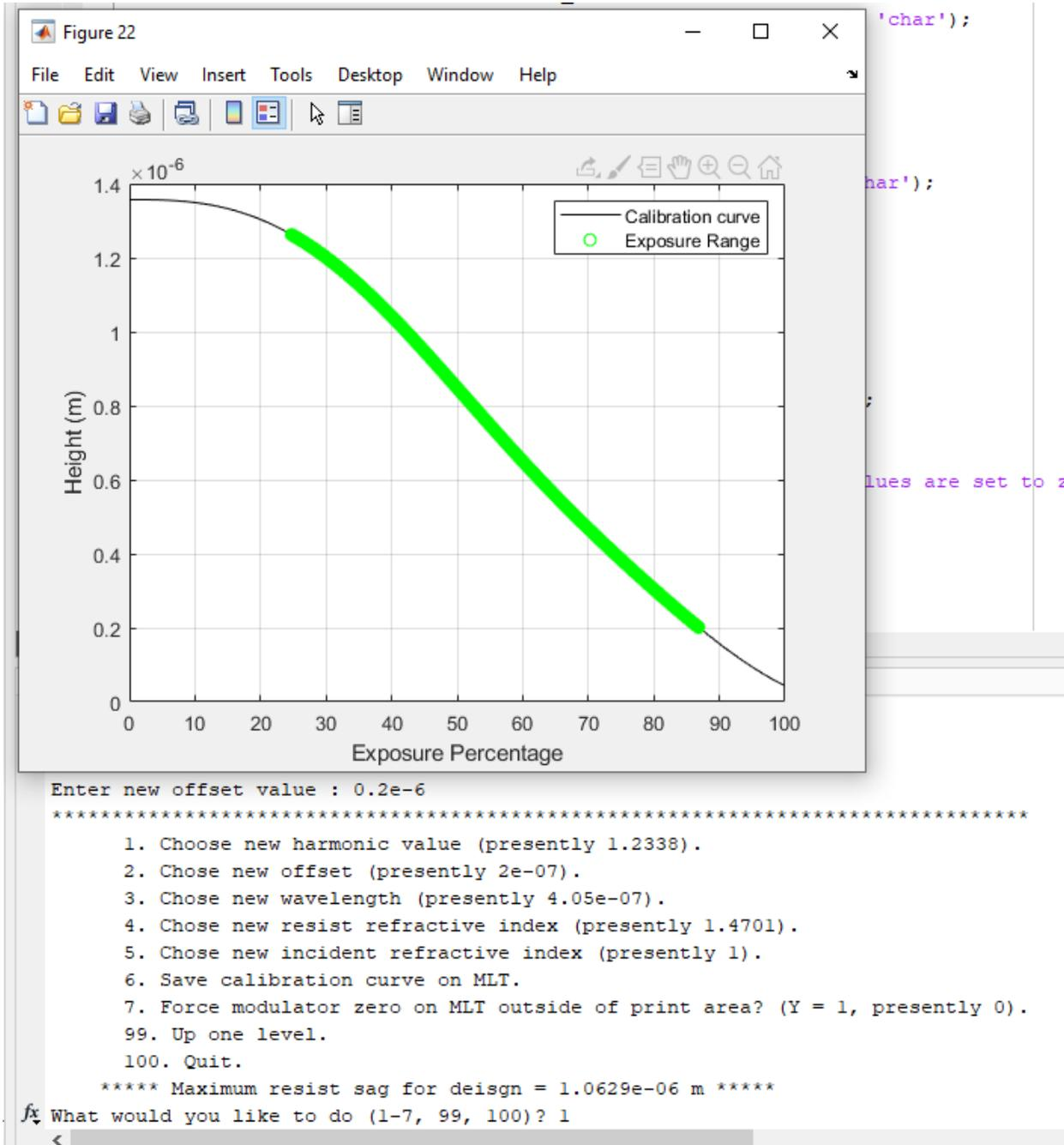
Figure 56 Resulting change on the location of the exposure range after changing the offset value.
