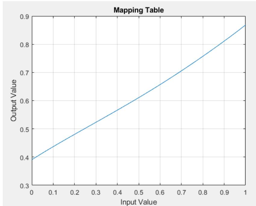
**Figure 59 Final Mapping Table output from the Linearization Process. The table correlates an original dose value (x-axis) with a calibrated dose value (y-axis)**
