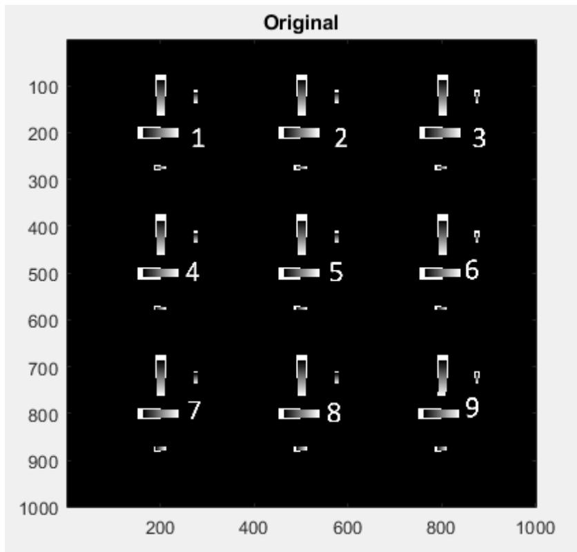
**Figure 26 Calibration ramp design via OptiScan. All ramp groupings are numbered to ensure similar features are compared when experimenting with different exposure parameters.**
