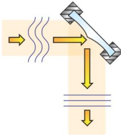
**Figure 3 Deformable mirror with a correction map applied manipulates a distorted incident wavefront [8].**
