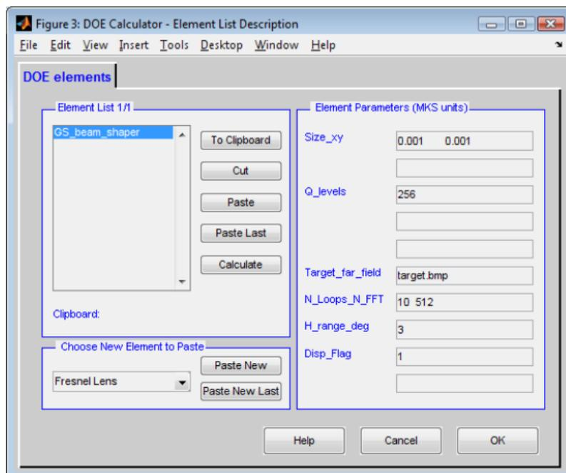
**Figure 24 DOE Elements window specifying the Gerchberg-Saxton beam shaper as an element**
