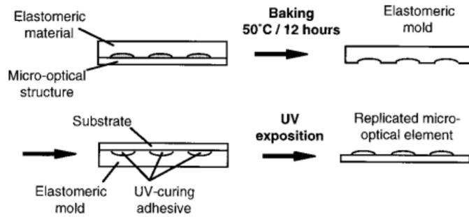
**Figure 9 Replication of lithographic exposure using elastomer molds and optical adhesive [13].**
