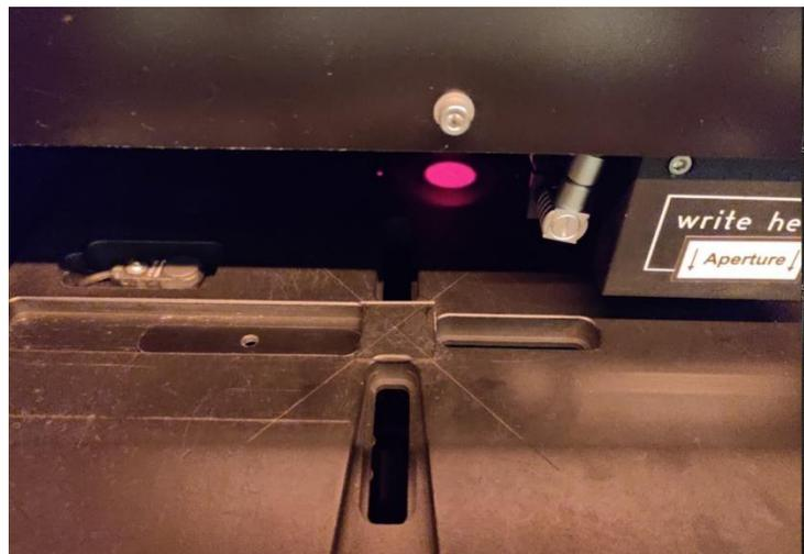
**Figure 13 Mounting sample to vacuum chuck in the loading area of the MLA 150.**
