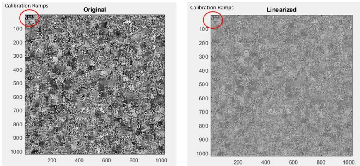
Figure 39 Original and Linearized CGH design for applications in adaptive optics for single shot phase retrieval
