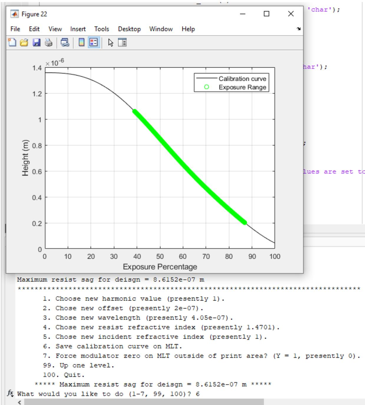
Figure 57 Choosing a new harmonic value. The exposure range is now correctly positioned.
