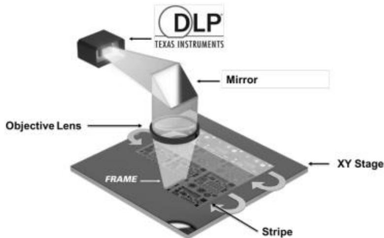
Figure 12 Depiction of raster-scan used by the MLA 150 to write patterns onto a substrate [4]
