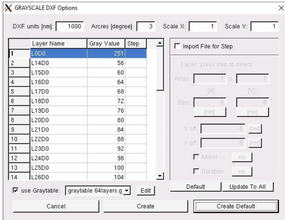
**Figure 14 Utilization of a gray table when converting a file for grayscale exposure for the MLA 150.**
