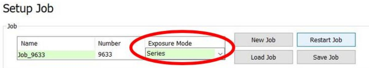
**Figure 18 ‘Series’ exposure mode being chosen in the Job Setup menu on the MLA 150 in order to perform a dose series test on a given photoresist**
