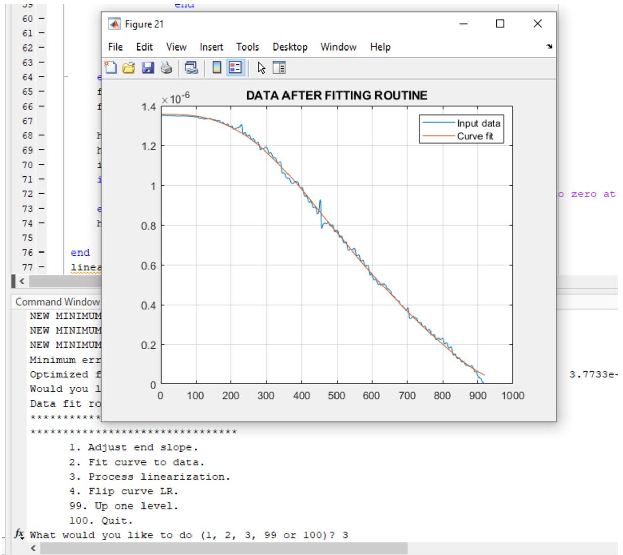
**Figure 54** Curve fitting routine complete, selecting option 3 to move on and process the linearization.
