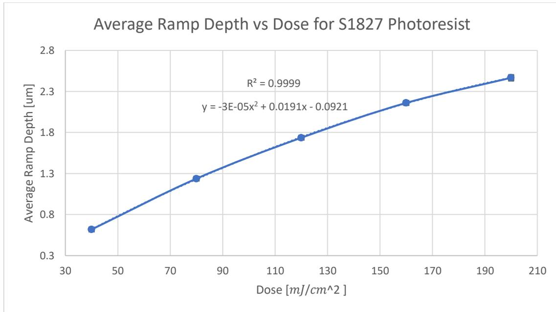
**Figure 22 Average ramp height vs dose plotted using the data shown in Table 4. A quadratic trendline is plotted with equation and R squared value shown. Error bars show +/- one standard deviation of the data set though they are insignificant and do not display on the graph.**
