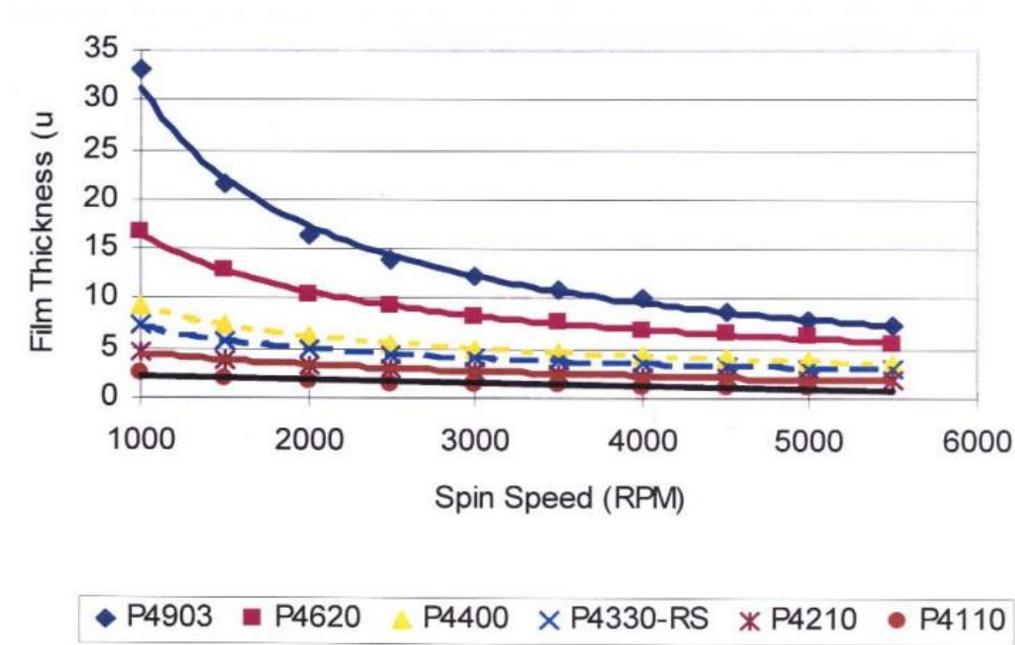
Figure 16 Spin speed curve for the AZ P4000 line of photoresists
