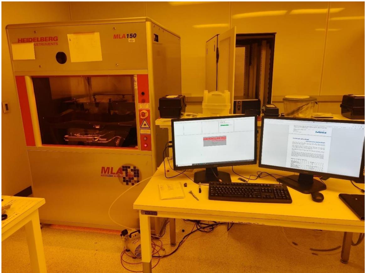
**Figure 11** MLA 150 housed in the 8<sup>th</sup> floor cleanroom of the Wyant College of Optical Sciences.
