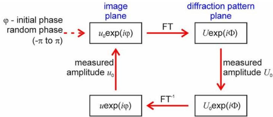
**Figure 7 Iterative phase retrieval methods of the Gerchberg-Saxton algorithm. FT denotes Fourier Transform [9].**
