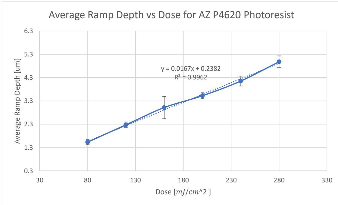
**Figure 23 Average ramp height vs dose plotted using the data shown in Table 5. A linear trendline is plotted with equation and R squared value shown . Error bars show +/- one standard deviation of the data set.**
