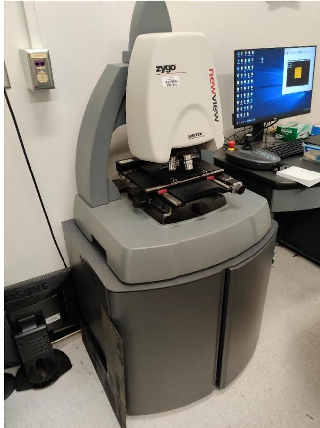
**Figure 17 Zygo NewView® 8300 white light interferometer housed in the Wyant College of Optical Sciences**
