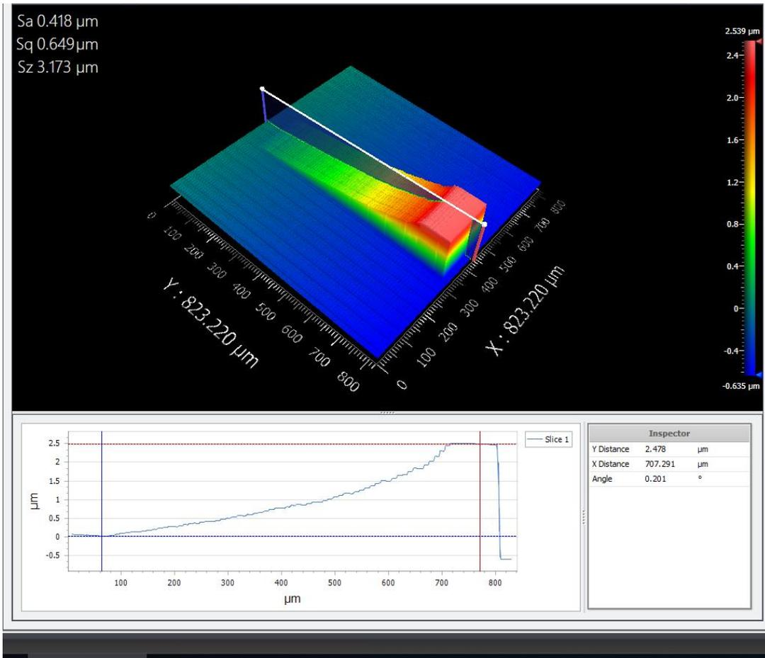
**Figure 27. Profile scan of a calibration ramp exposed with S1827 photoresist prior to being calibrated and linearized.**
