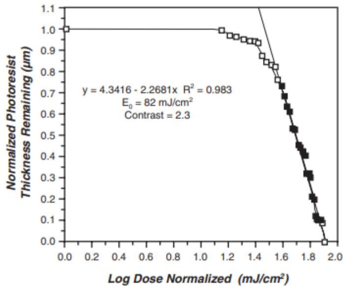
Figure 15 MICROPOSIT S1813 Photoresist Contrast Curve [17] .
