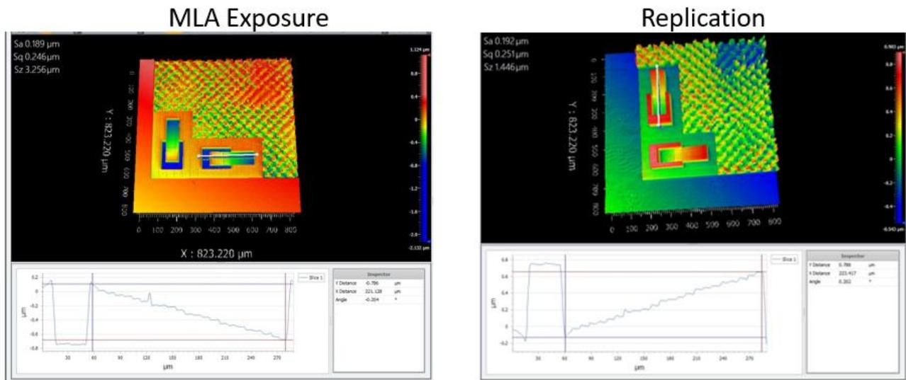
**Figure 40 Comparison of a similar feature (calibration ramp) of the original linearized exposure and the replicated element. The depth of the MLA Exposure ramp (0.786um) is very similar to its replication (0.788um).**
