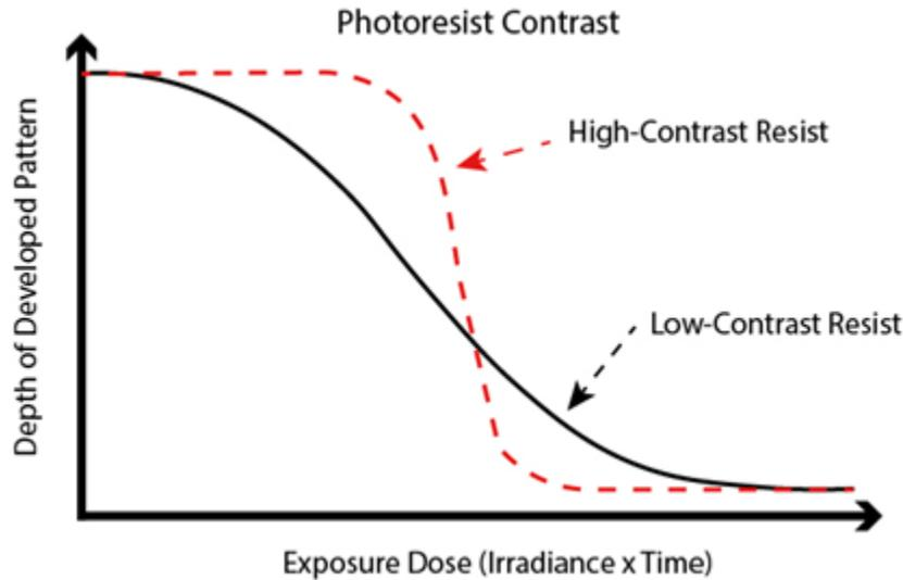
**Figure 1** Chart demonstrating the response of different contrast photoresists when an increasingly higher dosage of light energy is used. Binary applications utilize a high-contrast photoresist, where there is a steep curve from minimum to maximum depth that occurs over a small dosage range. Grayscale applications utilize a low-contrast photoresist, which are characterized by a gradual change in depth over a large dosage range [3].
