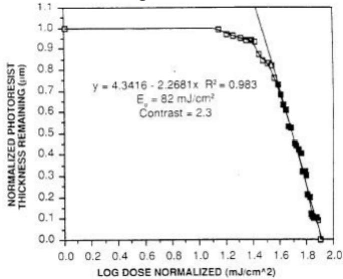
Figure 61 Normalized photoresist thickness vs. normalize dose (log) for S1813 photoresist.
