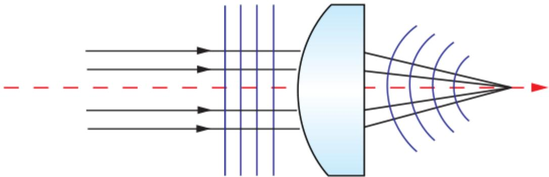
**Figure 2 Positive lens manipulating an incident planar wavefront into a converging spherical wavefront [8].**
