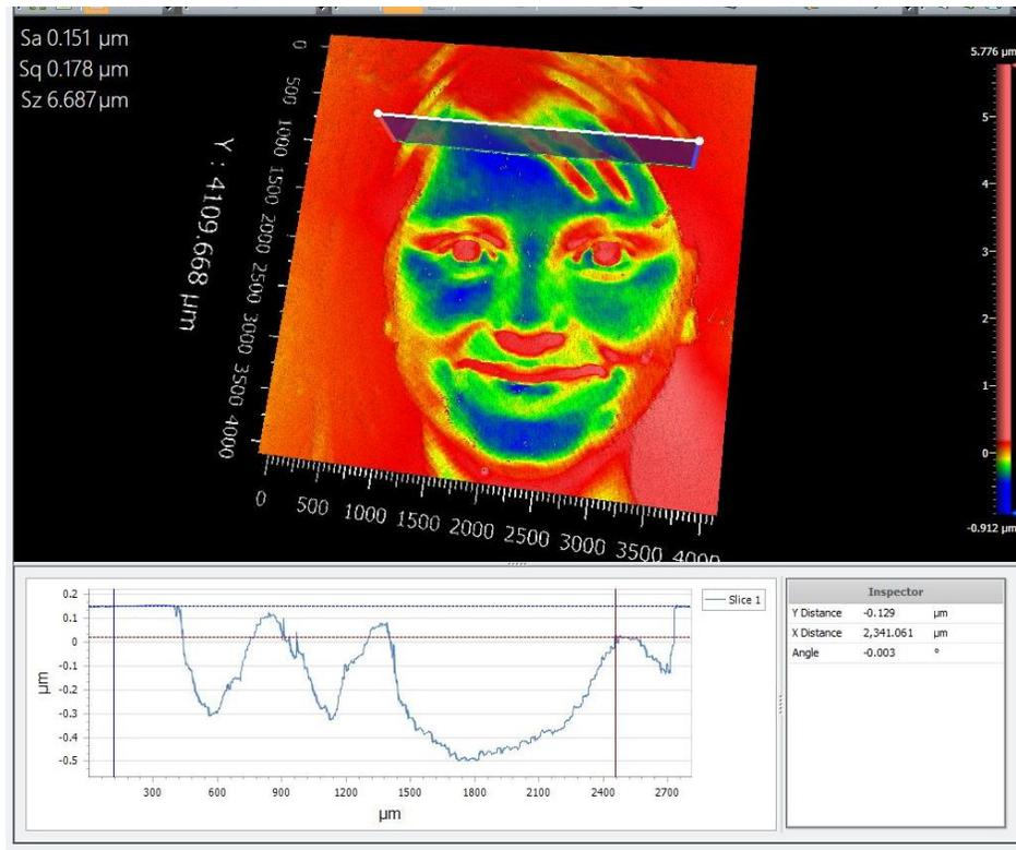
**Figure 36 Linearized exposure of a person's image in order to test the usage of a large and complex file. The profile shown is not significant, except to demonstrate the grayscale characteristics of the exposure. 4x4 stitched image using a 10x magnification objective.**
