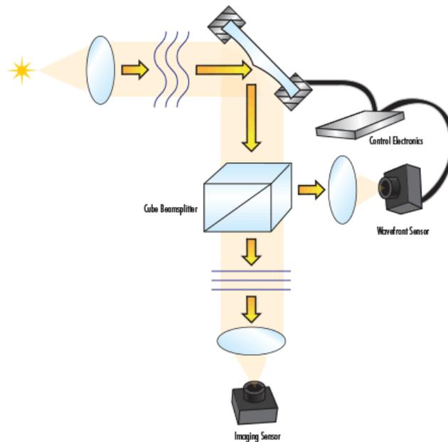
**Figure 6 Closed looped AO system utilizing a wavefront sensor to provide feedback to a deformable mirror [8].**
