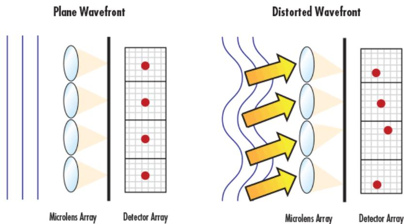
**Figure 5 Interaction between an incident wavefront and the lenslet array and detector plane of a Shack Hartmann Wavefront Sensor [8].**
