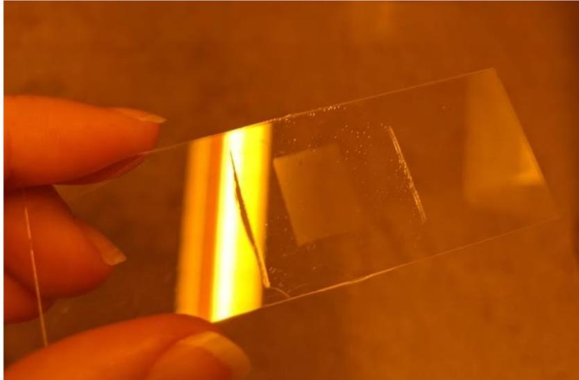
**Figure 38 Example of a replicated element with an 8X10mm diffractive pattern on a microscope slide.**
