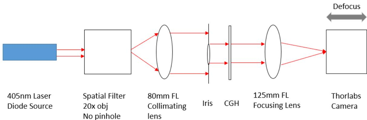
Figure 42 Diagram of CGH testbed with labeled components and light path
