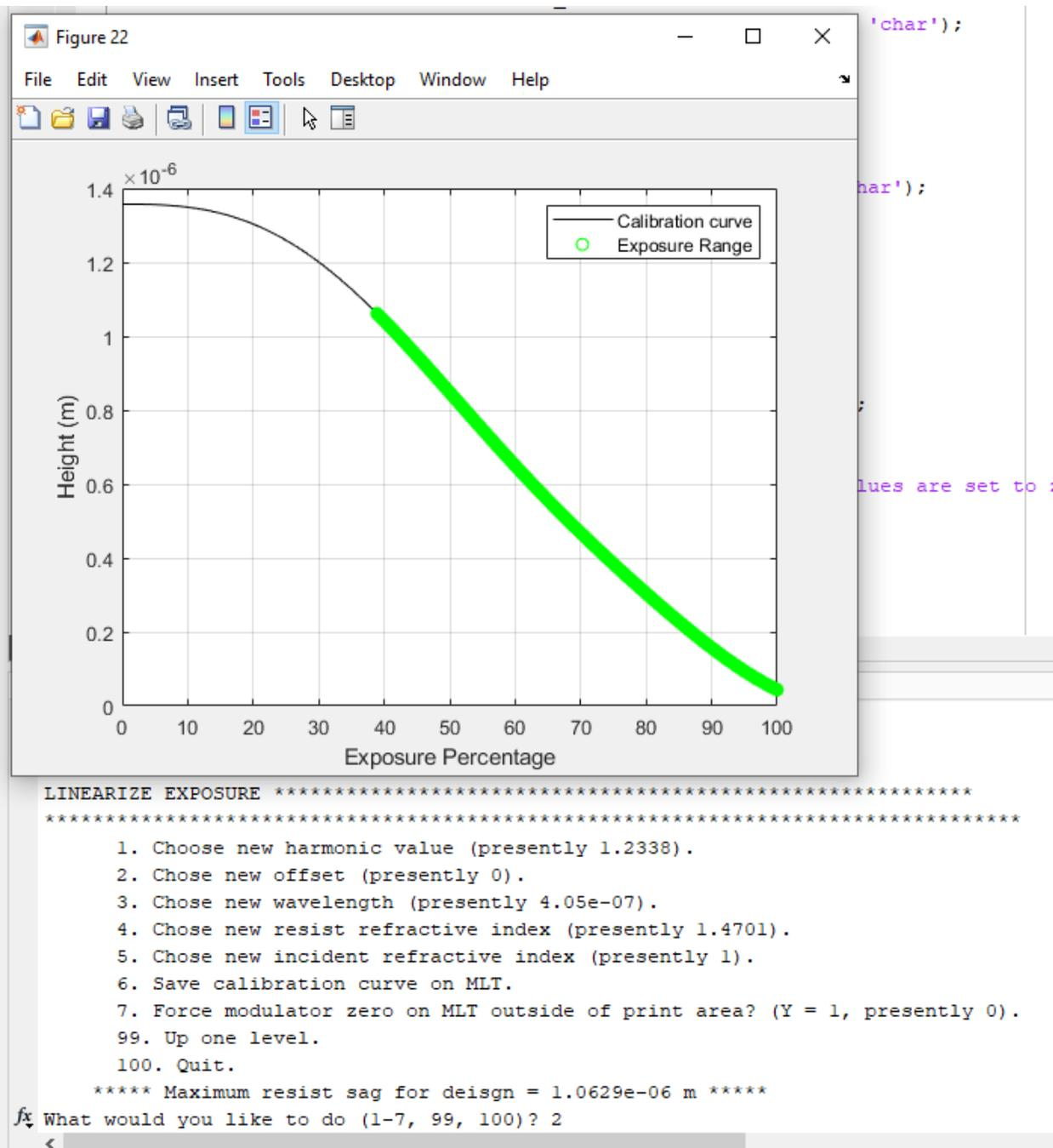
Figure 55 Initial processing of the linearization given curve fit data.
