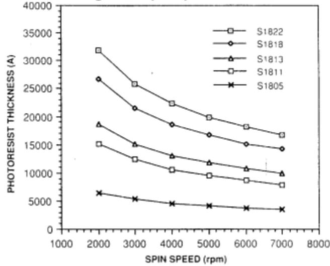
Figure 60 Photoresist thickness vs. Spin Speed for the S1800 series photoresist. S1813 and S1827 photoresists are included.
