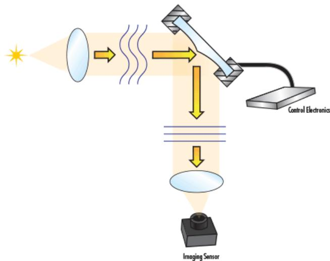
**Figure 4 Simple AO imaging system operating under open loop control [8].**
