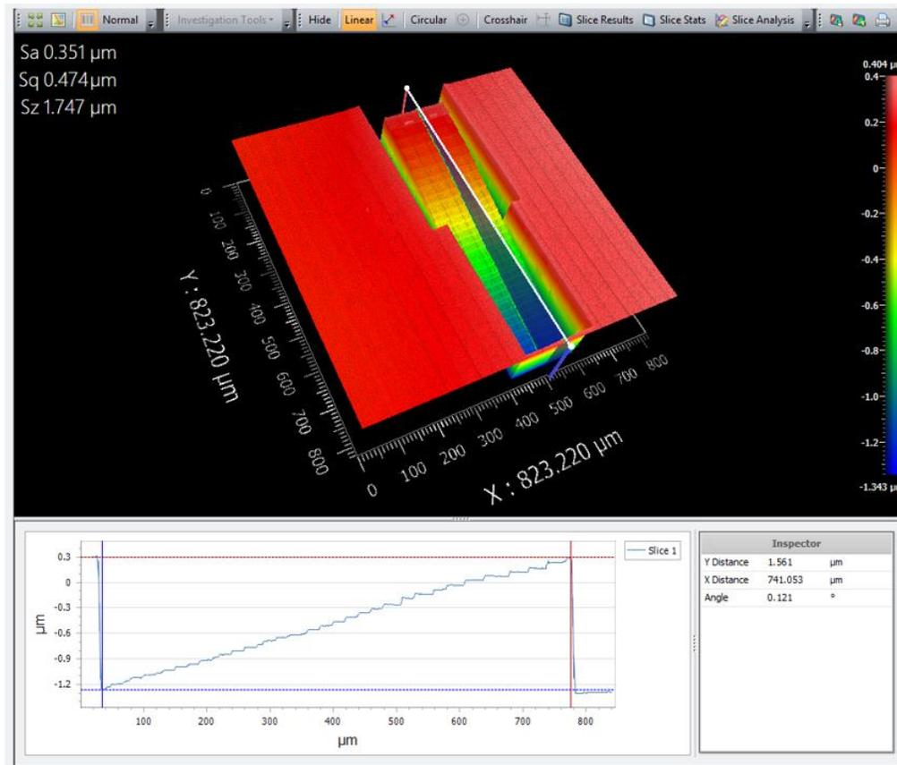
**Figure 33 Resulting performance of linearization on the calibration ramp pattern, comparable to the feature shown in Figure 27 that was measured before a linearization regime was applied.**
