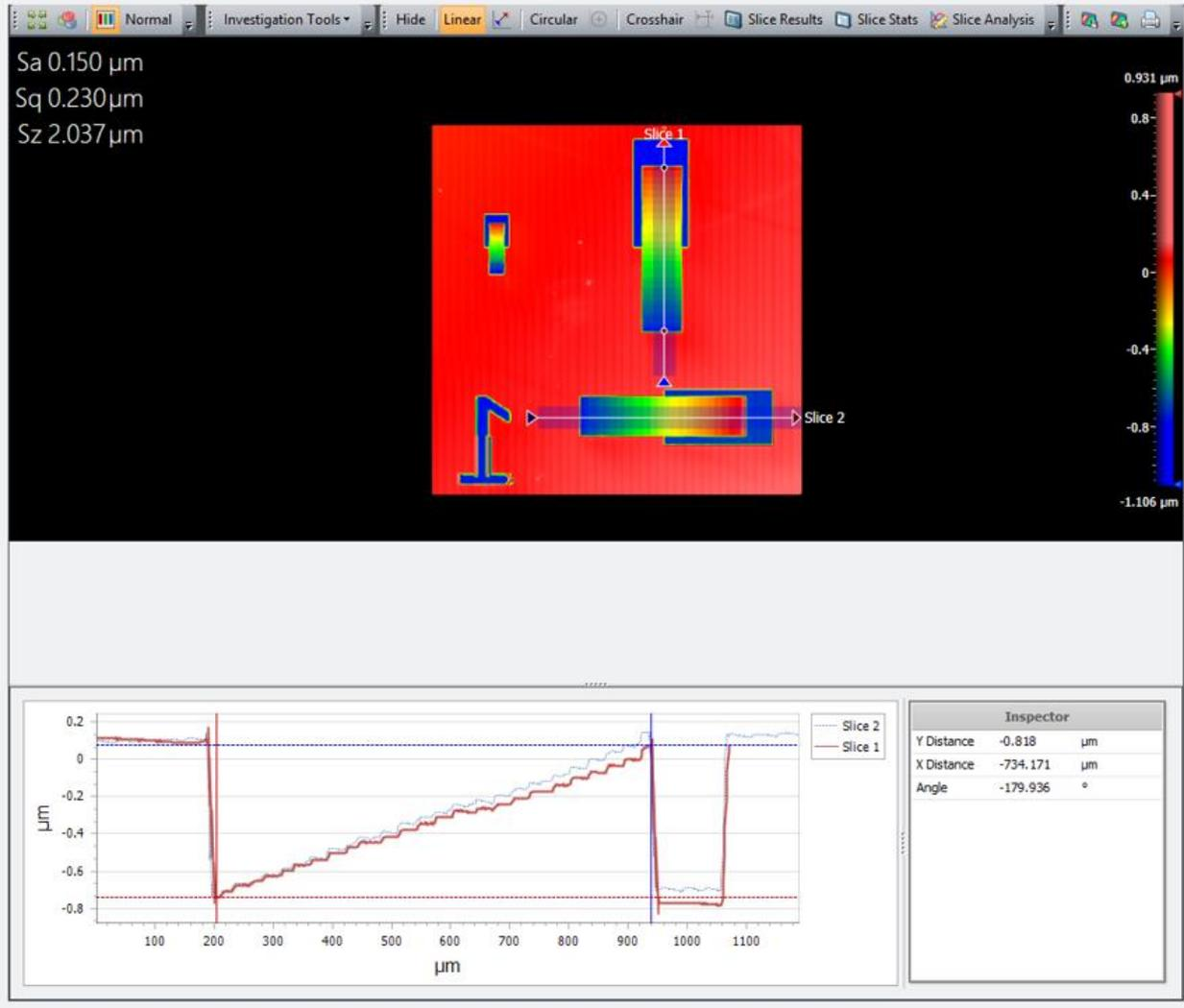
**Figure 34** Verification of linearized MLA exposure of the calibration ramp pattern over the x- and y- axis. The average profile of two 100 $\mu\text{m}$  thick slices are shown overlapping.
