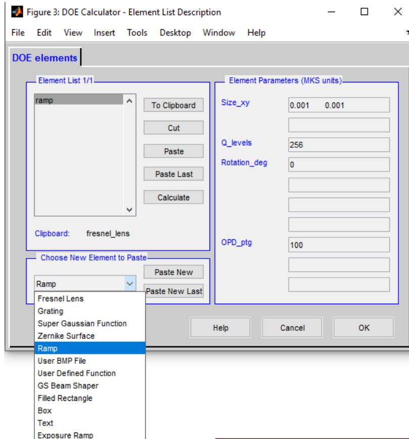
Figure 47 Adding a Ramp element to the Element List
