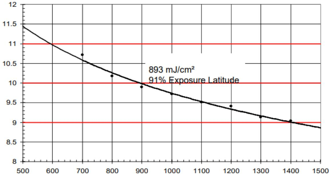
Figure 62 AZP4620 Lithography contrast curve. Photoresist depth vs. Dose
