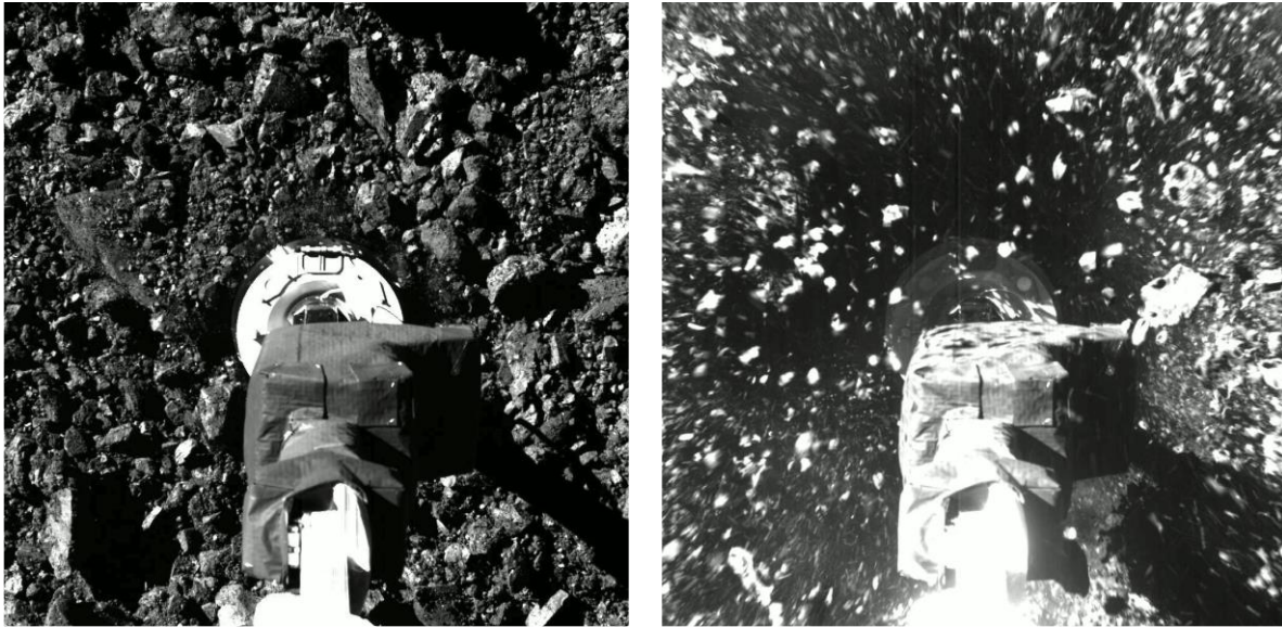
Fig. 9, Images of the Actual Sample Collection Event Taken Before Contact (left) and After (right).
