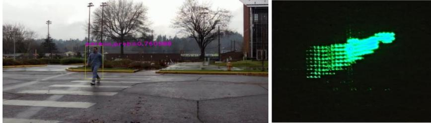
Figure 6. (a) A pedestrian walking across the road is captured by video camera. (b) CGH is calculated on-the-fly by to scan the angular extent and position of the pedestrian (Movie is available on archived presentation).
