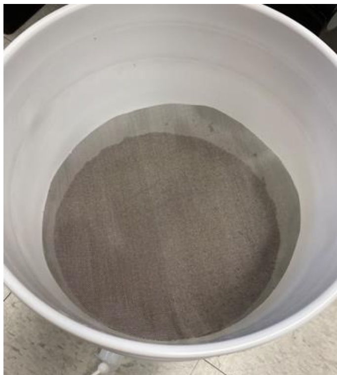
Figure 3. Screen on top of coarse sand in bottom bucket
