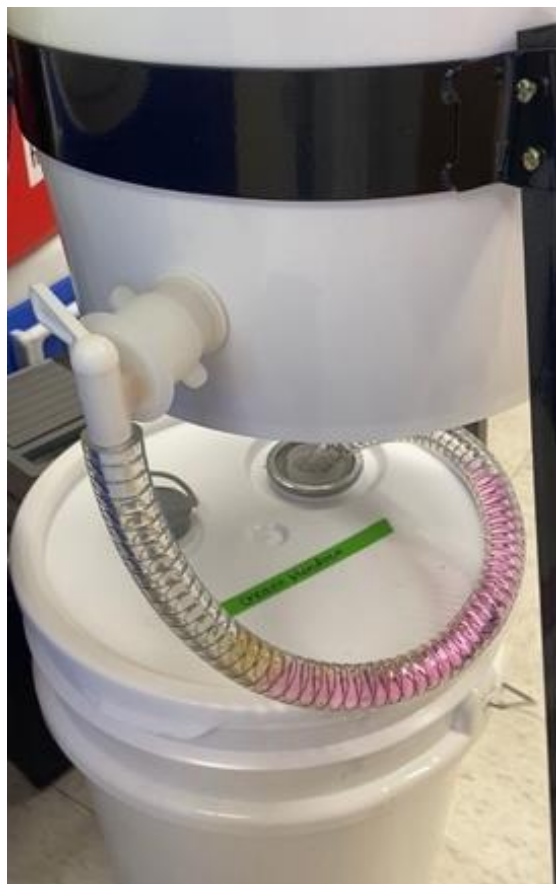
Figure 4. PVC tube facilitating flow of water into the bottom bucket
