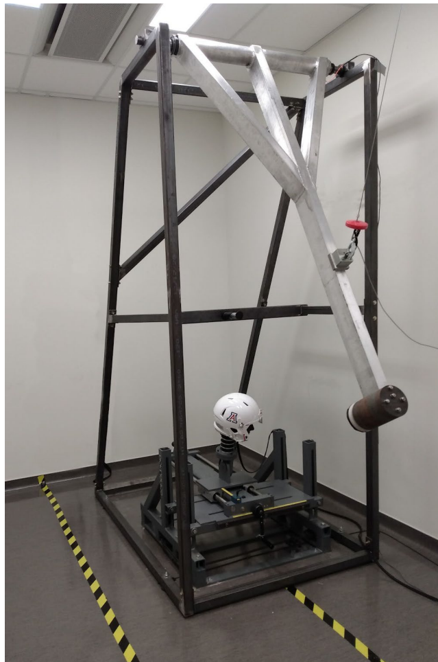
Figure 5: Assembled impact test device.
