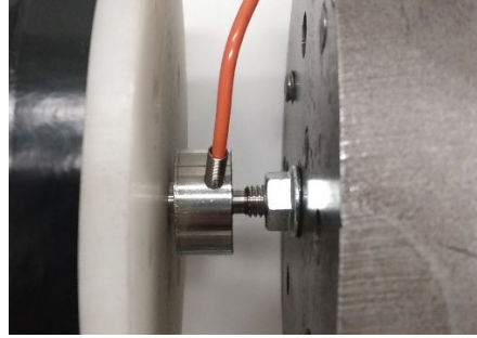
Figure 7: Load cell placement on impactor between endcap and steel plates.
