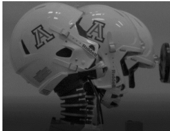
Figure 8: Overlay of high-speed video stills to capture the motion of the head throughout impact
