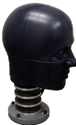
Figure 3: NOCSAE head form on Hybrid III neck
