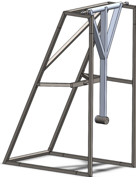
Figure 1: SOLIDWORKS® rendering of the complete pendulum design.
