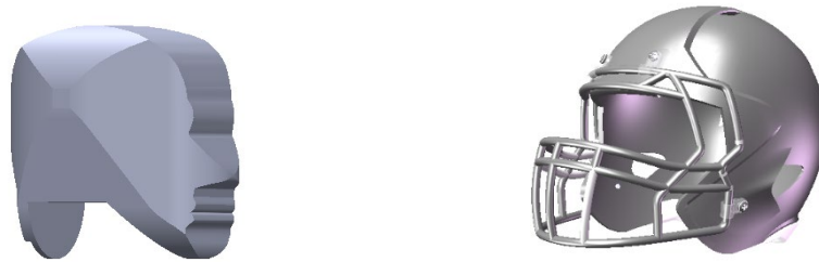
Figure 19: Surface geometries used to define impact location points. SOLIDWORKS renderings. Helmet geometry from [42].
