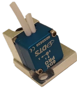
Figure 6: a) DTS 6DX Pro on custom mount
