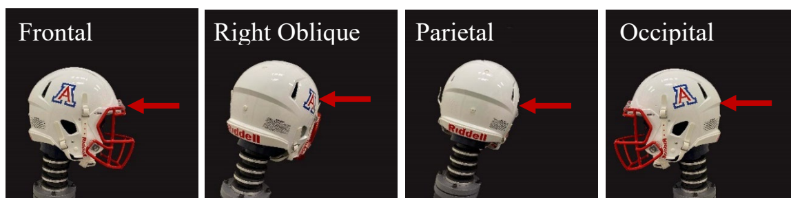
Figure 11: ATD orientation and location of impact.
