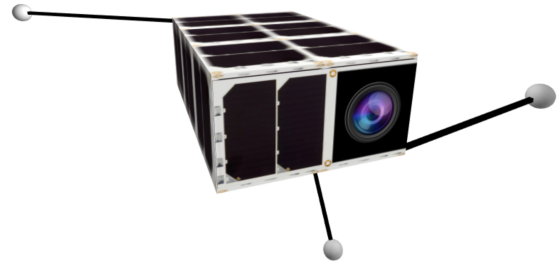
Figure 1. Proposed architecture for a 6U CubeSat space telescope. Each boom has a single degree-of-freedom in linearly independent axes, enabling three-axis attitude control. Magnetorquers are used to desaturate the angular momentum of the booms and keep them within their operating limits.
