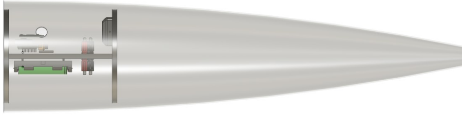
Figure 10: Telemetry Bay CAD Model Showing Location In Nosecone
