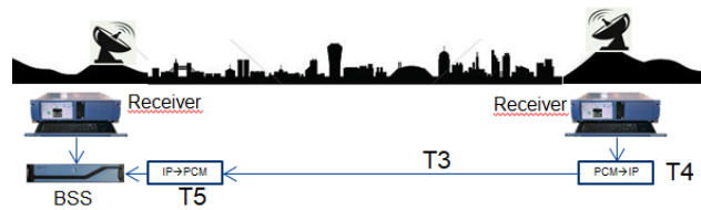
Fig. 2. Example of additional propagation time related to the distance between the antennas and the latency in the converters
