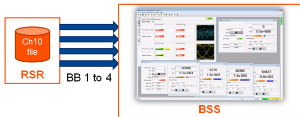
Fig. 12. Replay of the test signal into the Best Source Selector
