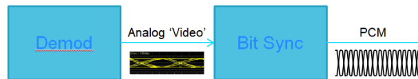
Fig. 5. Signal path in a receiver, showing that the signal quality available on the Analog “video” is lost in the PCM signal
