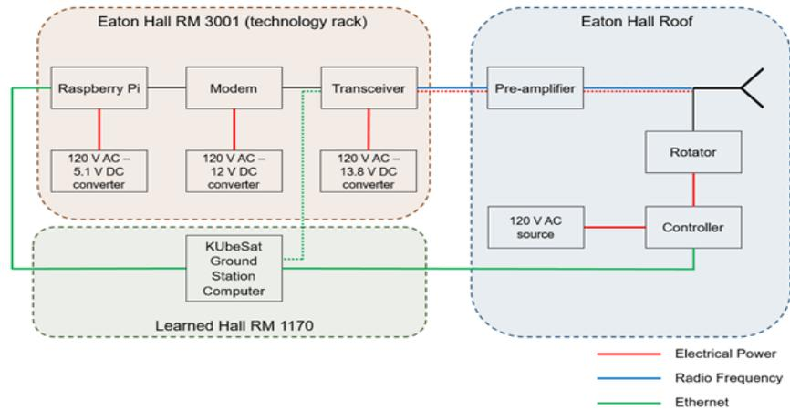
**Figure 2 Ground Station Block Diagram.**
