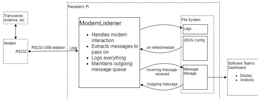
**Figure 4 Ground Station Software Infrastructure.**
