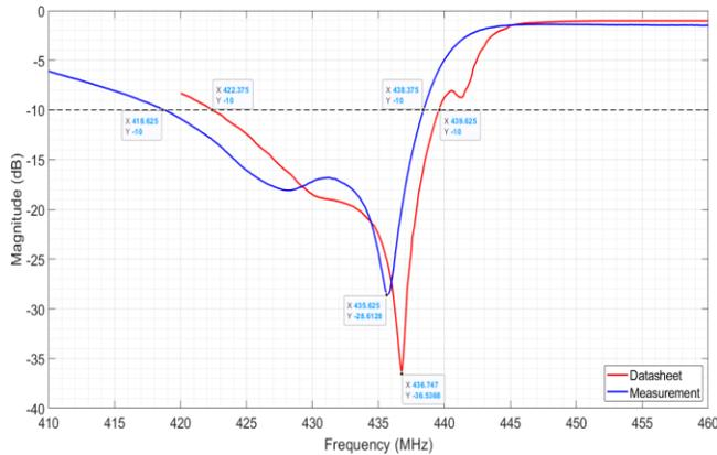
**Figure 5 Simulated and Measured Return Loss.**
