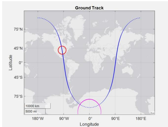
**Figure 1 KUBeSat-1 Ground Track for 1 Orbit at 550 km Altitude.**
