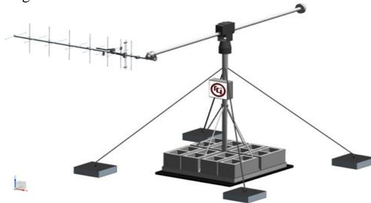
**Figure 3 CAD Rendering of Fully Assembled Ground Station.**
