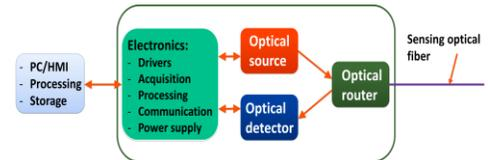
Fig. 8: Block diagram of fiber optic sensor interrogators
