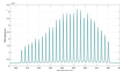
Fig. 16: FBG spectrum at 808-880nm
