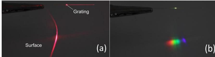
Fig. 11: a) red diode laser, b) white light LED imaged on a flat surface from a chirped first order PbP processed fiber-integrated diffraction grating by femtosecond laser pulses.
