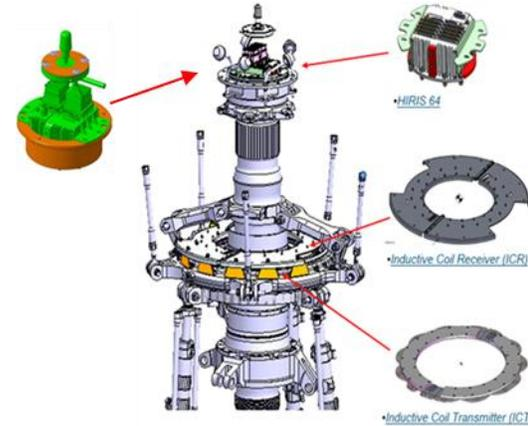
Fig.2: HIRIS installation scheme for the main rotor
