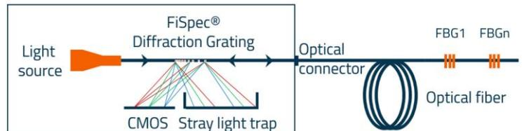
Fig. 12: Schematic illustration of a patented [4] FBG Interrogator around a single monolithic optical fiber.
