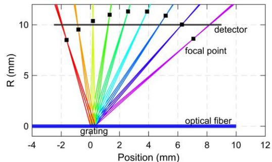
Fig.10: Simulated directions of constructive interference of two neighboring points at the beginning, the middle and the end of an aspheric chirped grating
