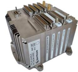
Fig. 17: XMA-ROTOR with 2 FBG interrogators + 5 other modules
