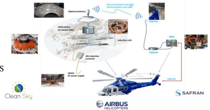
Fig.6: HIRIS prototype mounted on H175 main rotor
