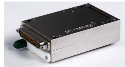
Fig. 15: 1<sup>st</sup> aerospace grade FBG-Interrogator prototype supply
