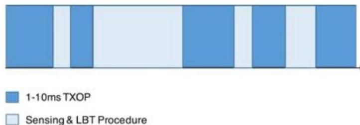
Figure 3 LAA LBT Waveform.<sup>1</sup>
