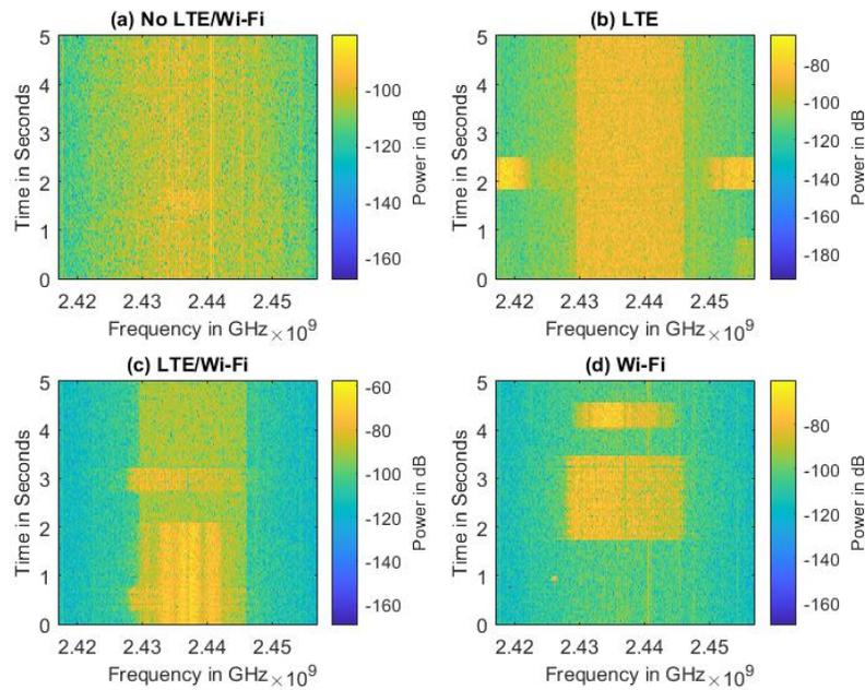
**Figure 7 Spectrograms of LTE/Wi-Fi coexistence testbed data.**
