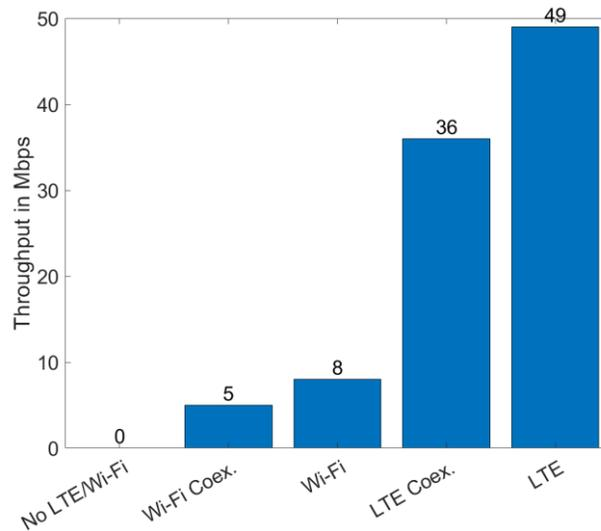
Figure 8 Throughput measurement in different scenarios.
