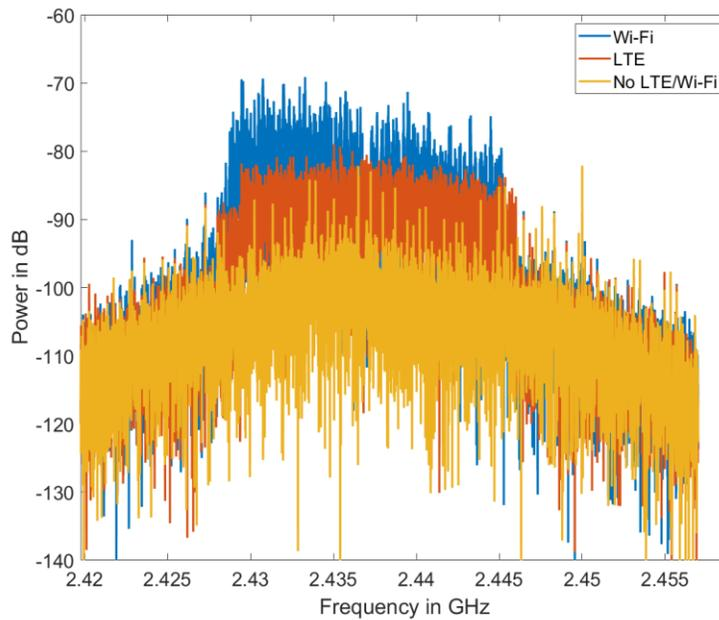
**Figure 6 Superimposed PSD of LTE-U and Wi-Fi.**
