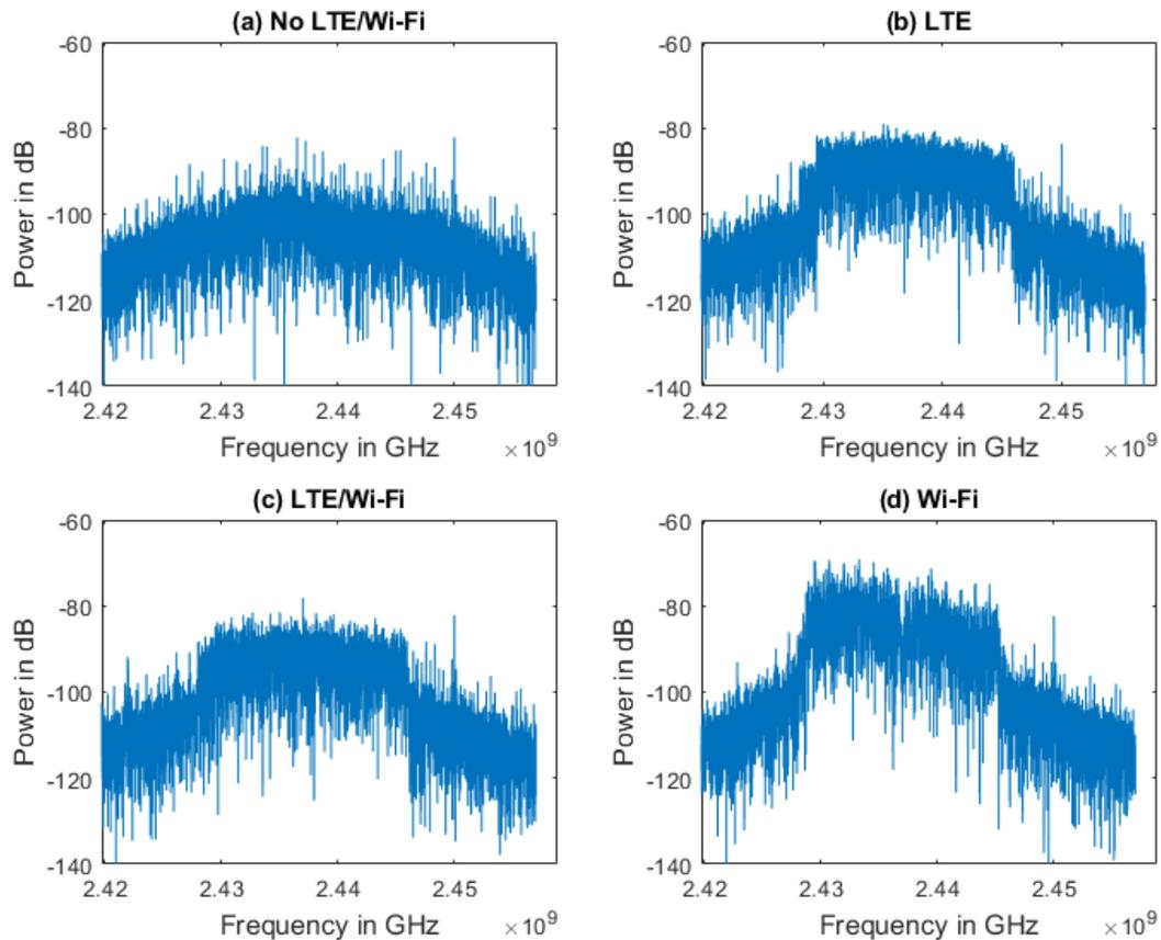
Figure 5 PSD of LTE/Wi-Fi coexistence.
