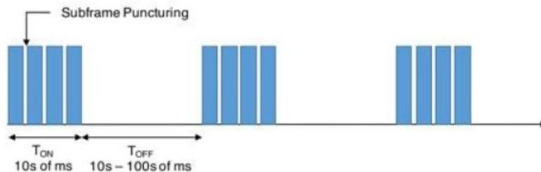
Figure 2 LTE-U waveform duty cycle.<sup>1</sup>
