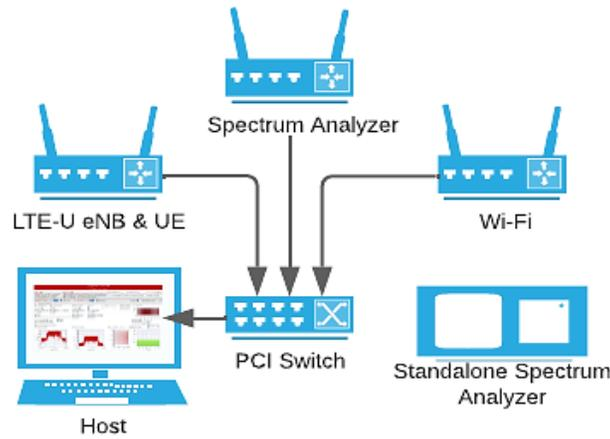
Figure 4 LTE/Wi-Fi coexistence experiment setup.
