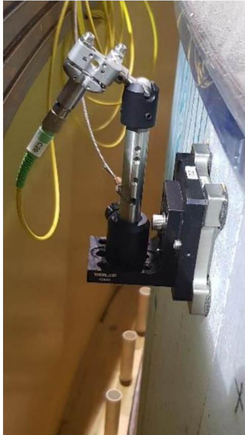
Figure 4-2. One of the 3.5 mm beam diameter collimators and its mount. The silver invar plate is bonded to the primary mirror wall. The plate contains magnets and provides a three-ball kinematic interface to the corresponding black mounting plate carrying the collimator. These collimator mounts, with a universal range of adjustment, were well suited for prototyping activities, where various geometries were being tried. A more dimensionally stable design is envisaged now as an upgrade path.
