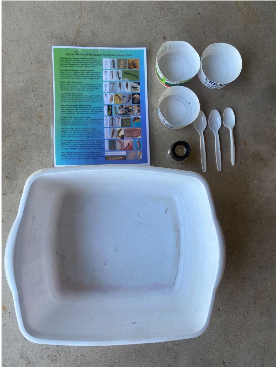
Appendix #1. Sampling gear used in field surveys including white plastic tub, smaller containers, and short field guide.
