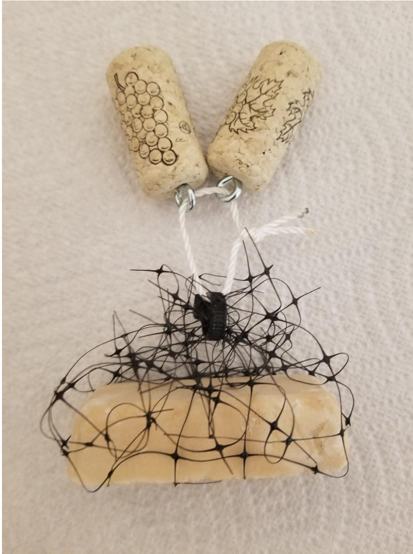
Figure 6: Float device containing a FourStar Bti briquet designed to keep the larvicide near the water level in which the larvae reside.
