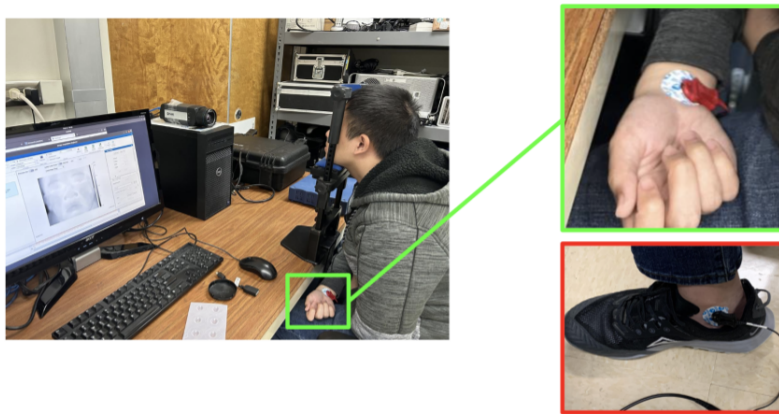
Figure 3: Experimental Setup . The left image shows the entire setup, the images on the right show placement of electrodes on subject for recording ECG. The red box illustrates electrode placement on the subject’s foot (out of view in the left picture).
