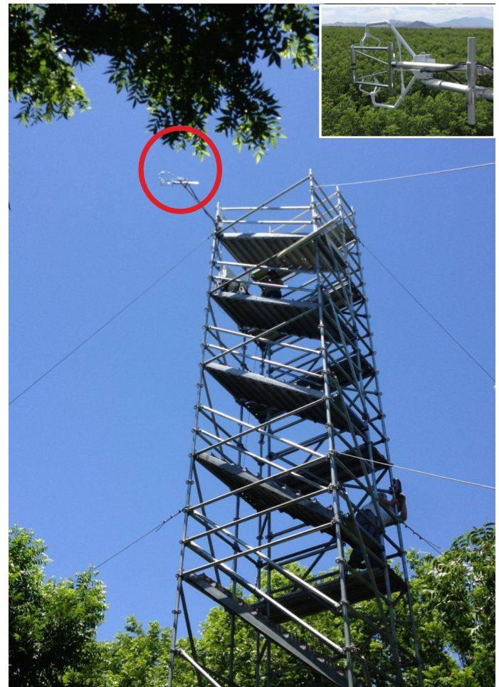
Figure 1. Walk-up flux tower that supported the eddy covariance instrumentation (red circle) used to measure pecan consumptive water use (CU). Inset photograph in upper righthand corner shows eddy covariance instrumentation.
