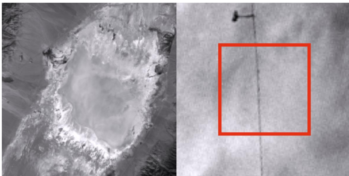
Figure 2. ASTER image of Railroad Valley (left) and 1 km 2 ROI (right), using the ASTER green band. The red box outlines the 1000 m × 1000 m RadCalNet ROI.
