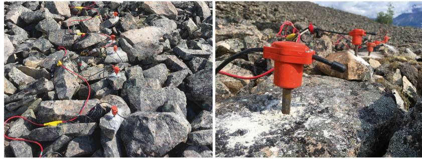
Figure 2. Method for geophone coupling to individual debris clasts after Maurer and Hauck (2007).
