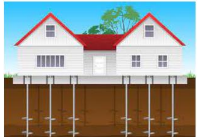
Figure 7. Illustration of Helical Pier System
