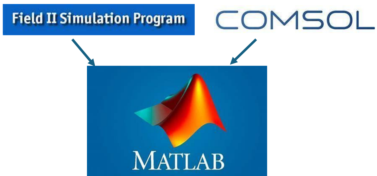
Figure 3: Ultrasound fields are simulated in Field II. Electrical and RF properties are simulated in COMSOL. These simulated properties are imported into MATLAB to then model the resultant AE fields and RF measurements. [4]
