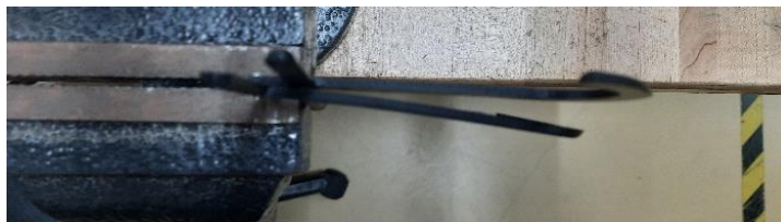
FIGURE 8. Bending of the hook after load test
