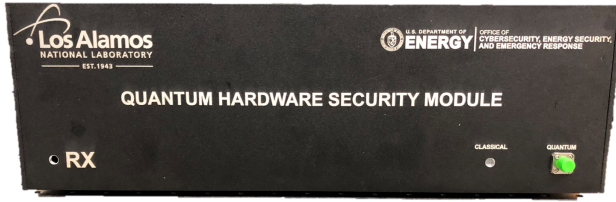
Fig. 2. Quantum Hardware Security Module (Q-HSM) designed and built at Los Alamos. Each Q-HSM device acts as a quantum key transceiver, with transmit and receive capability included. The transmitter comprises an attenuated laser that produces weak coherent pulses of light, with polarization per pulse set in one of four states. The receiver comprises an avalanche photodiode single-photon detector, optics for polarization analysis, and custom microelectronics for synchronization and control.
