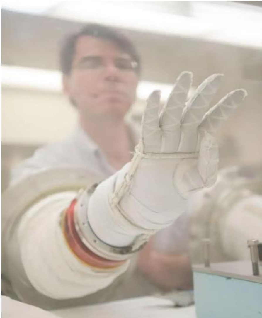
Figure 2 Astronaut Glove Challenge (2009) – An advanced astronaut glove prototype is tested in a vacuum chamber at Johnson Space Center in Houston, Texas. Its wearer, Peter Homer, won the challenge in both 2007 and 2009 image credit NASA
